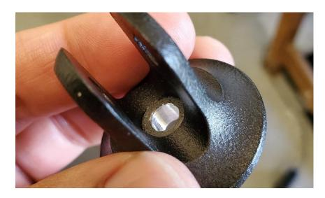
**2.20.** Using two low profile 25mm long SHCS, slide them through the top of the clevises and thread them into the rivet nuts just installed. Orient them parallel with the front of the car as shown, and torque to 6 ft-lbs.
