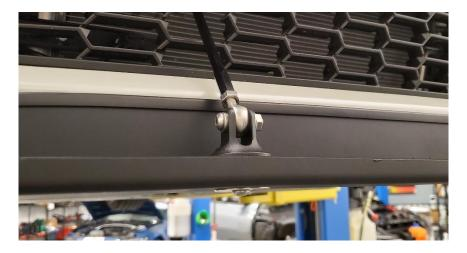
**2.37.** Use two 45mm long BHCS, fender washers, 15mm, and 5mm nylon spacers to bolt the splitter to the radiator support splash shield on both sides (the plastic cover with the metal U-nut). This is shown below.
