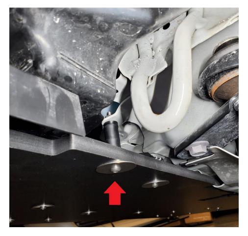
2.39. Finally, use two 40mm BHCS, fender washers, 5mm nylon spacer, 18mm washer, and M6 serrated flange nut to bolt the splitter to the last outer hole on the bumper (closest to the wheel well). You will need to push the fender liner to the side to get the nut and washer above the bumper as shown. BRZ Install Note: BRZ models do not have pre-drilled holes in these locations. Use the splitter blade as a template to drill a hole in this location using a ¼" drill bit, then install as written above.
