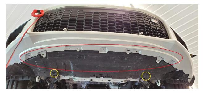
**2.5.** Next, we will remove the push clips that attach the fender liner to the bumper splash guard. Do this on both sides.
