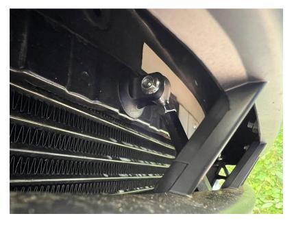
**2.32.** Re-install the radiator support splash shield with only the three bolts.
