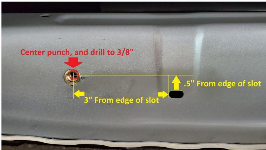
2.17. Once the holes are drilled to 3/8" touch up the raw edges with touch up paint.
