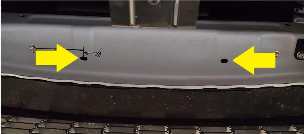
2.16. Measure from the edge of the slot 0.5" towards the rear of the car (towards radiator). From there, measure 3" outwards from the outer edge of the slot towards the side of the vehicle. Mark that point, and drill it to 3/8". Repeat the process for the opposite side. **Note:** Using a center punch before drilling is advised to ensure the drill bit doesn't walk.
