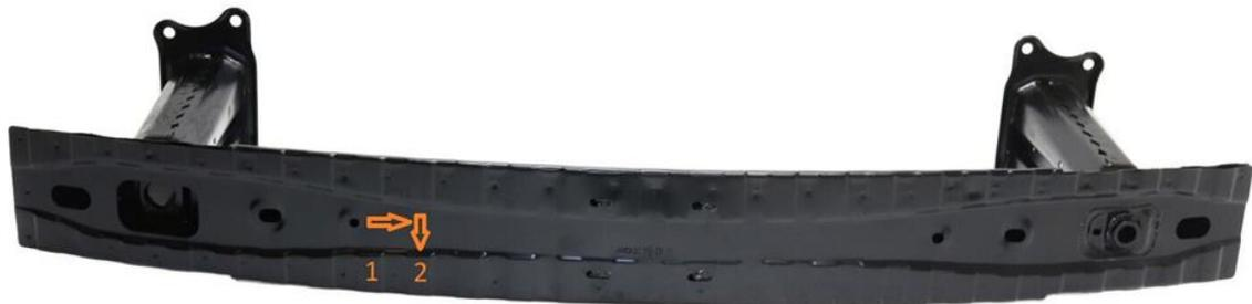
**2.26.** Drill both of these locations with a 1/4" drill bit. **Note: Using a center punch before drilling is advised to ensure the drill bit doesn't walk.**
