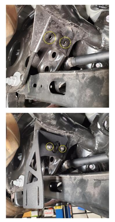
**2.5.** Locate, and remove the clips for the C-shaped bracket installation. The passenger side is shown below. The driver side is a mirror.
