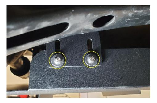
**2.8.** Install both side strakes onto the diffuser with eight 16mm long BHCS, 18mm washers, and M6 serrated flange nuts. Torque to 6 ft-lbs. The bolt heads, and washers should be visible from the outside.
