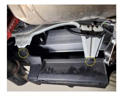
**2.6.** Next, install the C-shaped brackets using 16mm BHCS, 18mm washers, and M6 serrated flange nuts as shown below. The longer bracket is used on the outer location while the shorter bracket is used on the inner location. Make sure the side with the slotted hole is facing the ground.
