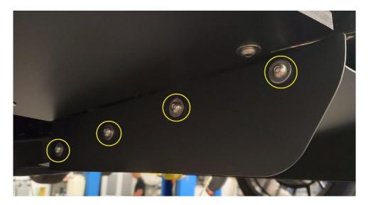
**2.9.** Next, figure out how high the diffuser can sit without making contact with the exhaust. Two lengths of bolts are supplied (25mm long and 45mm long), as well as an assortment of spacers so that this can be achieved.
