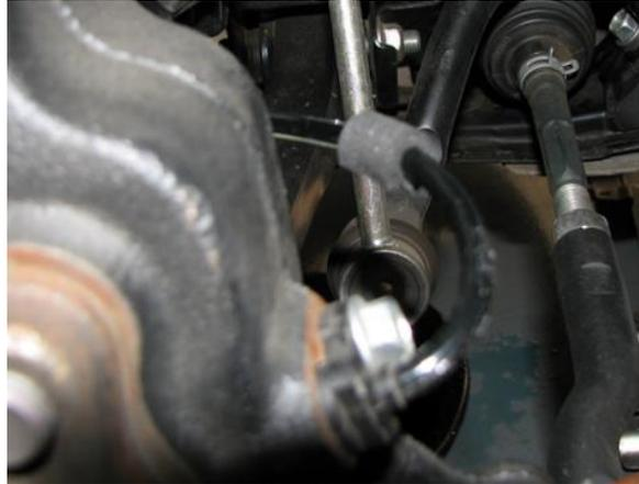
**2.12.3.** Reinstall the backing plate to ensure the foam is in the correct location. Below is a photo showing the foam tape protecting the wire as it is touching the carbon duct. The goal here is to have no movement and a snug fit to ensure the wire does not get abraded over time.
