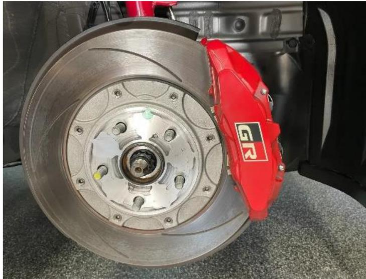
2.8. Remove the brake caliper by unbolting the 17mm caliper bolts.
