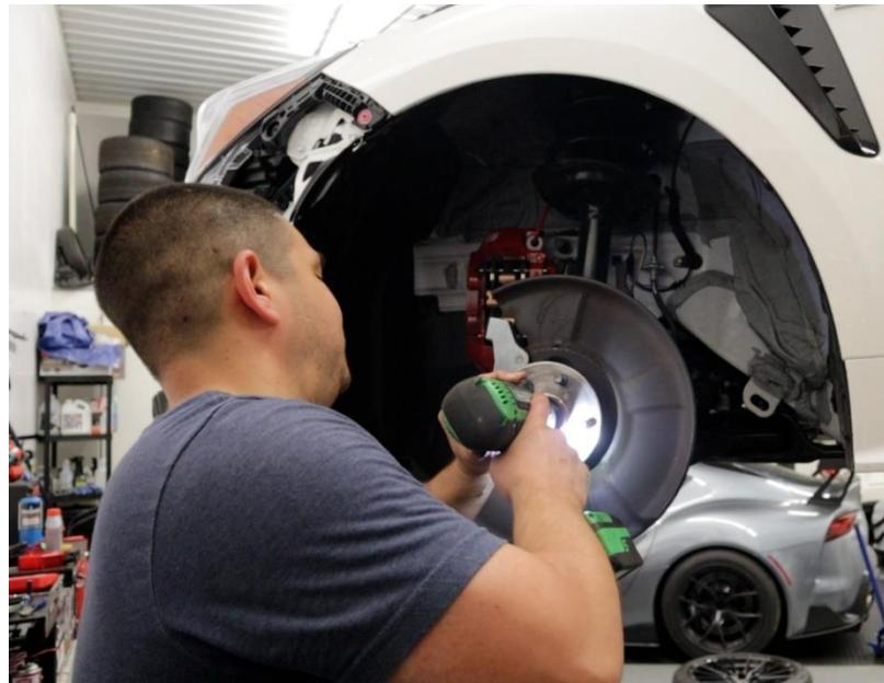
**2.11.** After the axle nut is removed, we now need to remove the hub assembly. Do so by using a combination of the 19mm wrench and 19mm socket with a 6" extension and swivel adapter.
