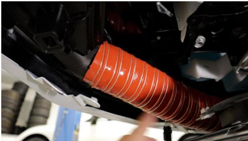
**2.13.1.** Next, route the hose under the washer fluid reservoir as shown below.
