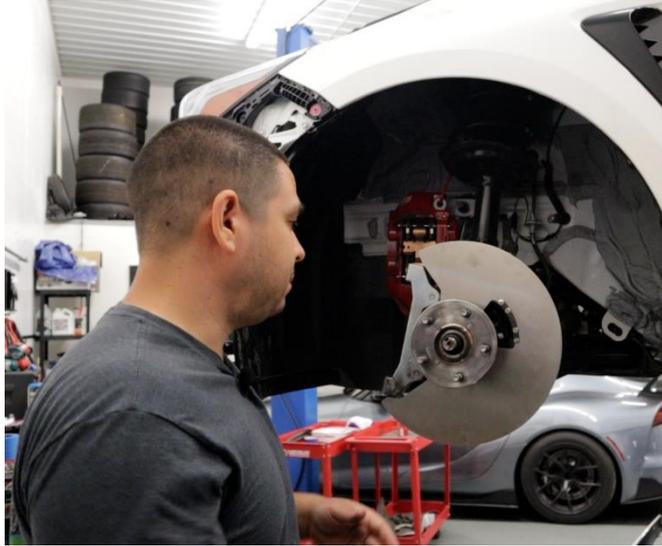
**2.12.5.** Install the axle nut and torque to factory spec. We highly advise replacing the axle nut after it has been removed, but depending on how new the car is, you might be able to get away with reusing the old axle nut. We opted for new axle nuts.
