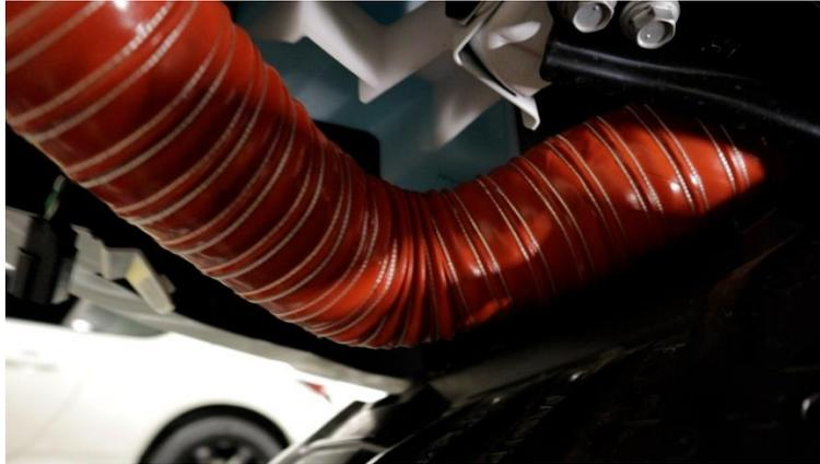
**2.13.2.** Continue routing the hose above the radiator support bracket and next to the charge cooler piping.
