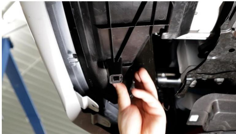
2.6.1. After you figure out where the tray is touching the ducts, use a utility knife, side cuts, dremel, or saw to trim the tray. Below is a photo of how much we removed.
