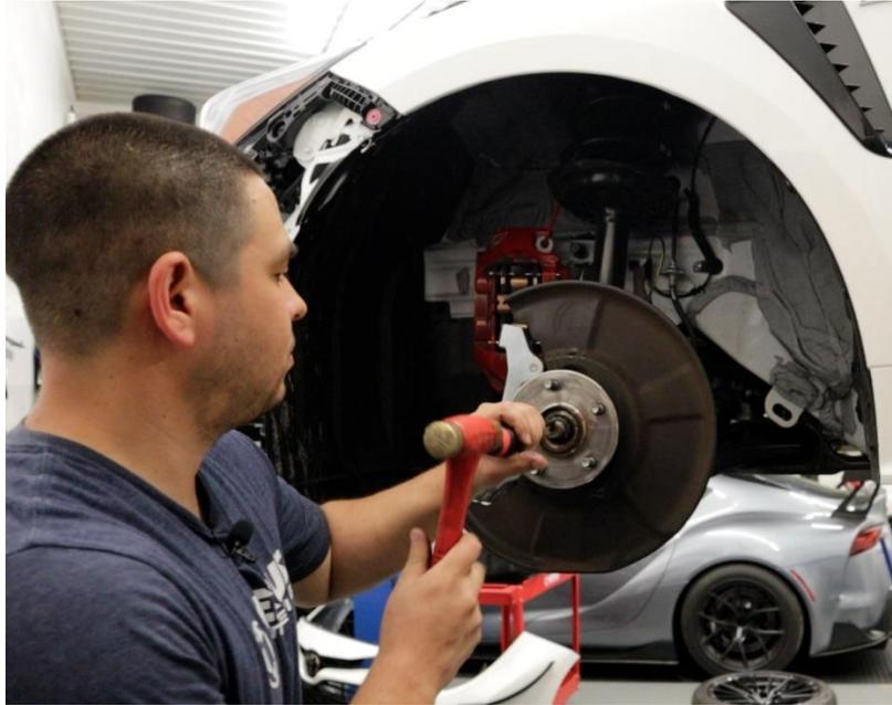
**2.10.1.** After the keyway is opened up, remove the axle nut using the 30mm socket and impact gun.
