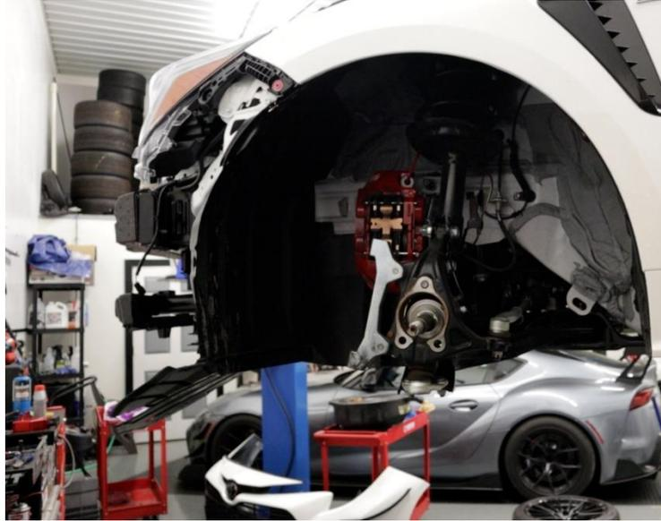
**2.12.** Now we need to install the backing plate kit. Start by using the hub mounting bolts for locating the backing plate. **Note: The carbon duct should face inward and should be towards the rear of the car as shown below.**
