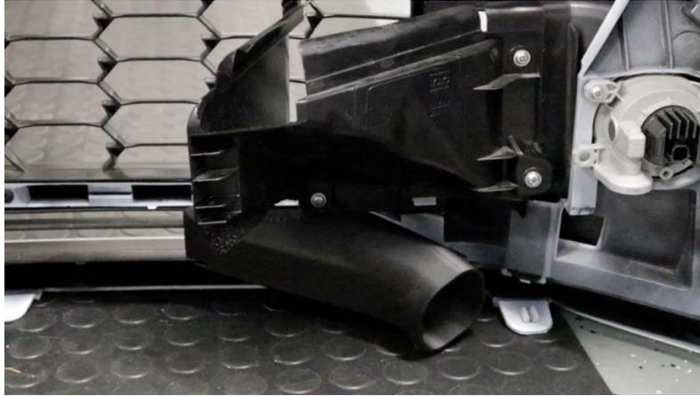
2.6. After the inlet ducts are installed, push the radiator support tray back in place to figure out where you need to trim it.
