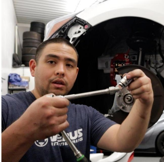
**2.11.2.** You might find that you need to free up the axle to gain more clearance for removing these bolts. To do so, thread the old axle nut back on until it is flush with the end of the axle. You may now tap it with your rubber mallet to break it loose. **Note: The older the car, the harder you will need to tap.**
