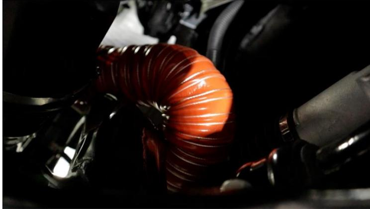
**2.13.5.** Finally route the hose above and parallel to the tie rod.
