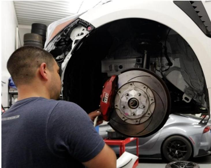
**2.8.1** Secure the caliper away from the hub assembly using caliper hangers, as shown below.
