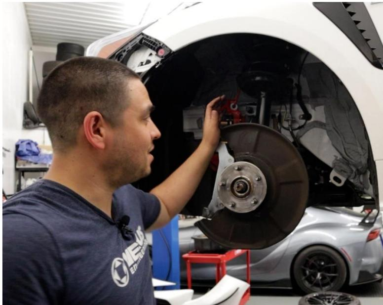
2.10. Now we need to remove the axle nut. Utilize a punch or a chisel and a hammer to un-stake the axle nut (the part that is crushed into the keyway, we need to push this up and out of the slot).
