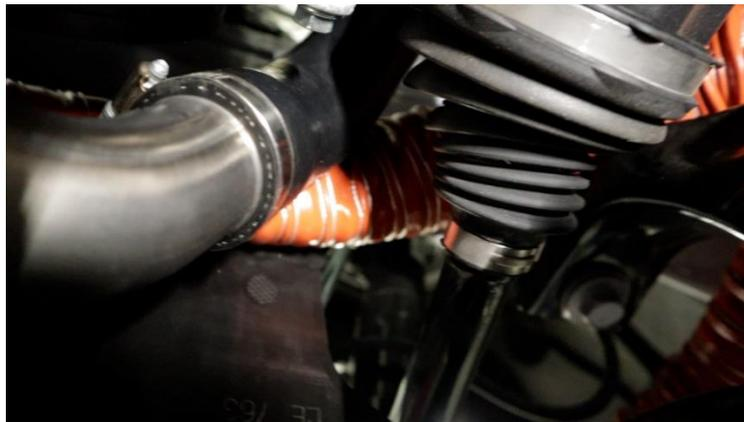
**2.13.4.** Route the hose around the mounting point for the sub-frame.
