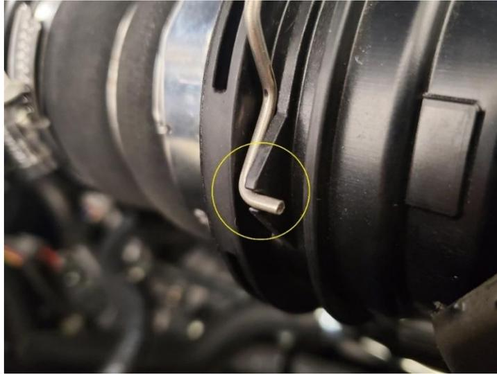
**2.3.2.** Remove the intercooler, and charge-pipe assembly.
