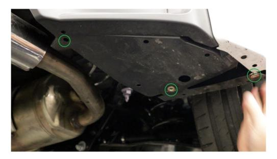
**2.5.** To properly install the rivet nut, you will want to thread the rivet nut onto the tool as shown below, and place the rivet nut into the hole.
