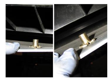
**2.8.** After the rivet nuts are installed, put the bumper cover back into place and install the rearmost push clip as shown below in orange.
