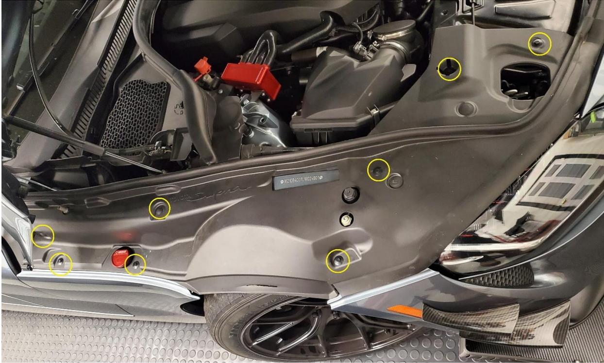
**2.10.2.** Remove the top two bolts. When removing the headlight bolts make sure to hold back the washer above the pink retainer. Again, marking the head of the bolts to ensure it is reinstalled in the same spot is a good idea.
