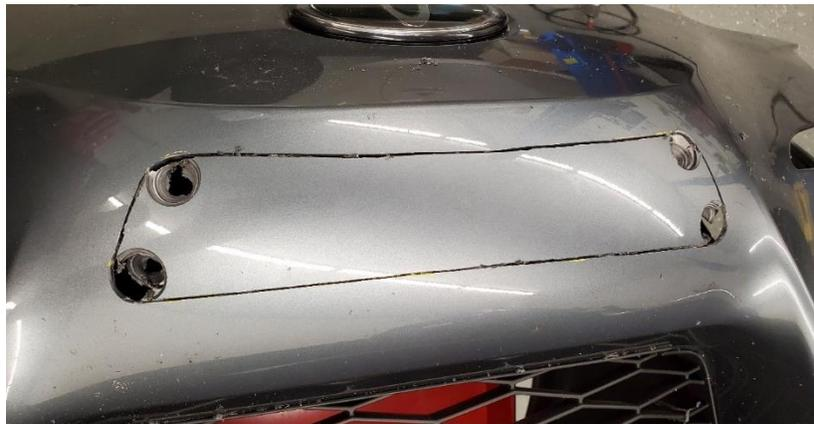
2.8. Using your cutoff wheel or air saw, cut out the hole for the Carbon Intake Inlet.
