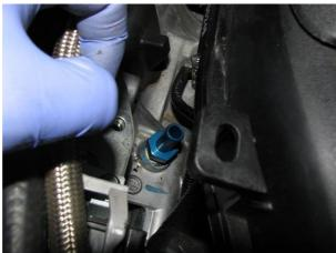
**2.9.** Remove the other side of the PCV system, which goes from the block (via a black plastic fitting under the A/C compressor) to the intake tube. It is the hose drawn in yellow and circled in yellow below. **It may be easier to remove the AC compressor, remove the belt and unbolt the compressor. We used 45 degree needle nose pliers.**
