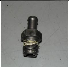
**2.8.** Install the supplied 3/8 NPT to 1/2" adapter fitting. You will need a 13/16" deep socket to install this. It is recommended to use some Teflon tape or sealant to ensure a leak free seal as shown below. Install this adapter to 12-18 ft-lbs.
