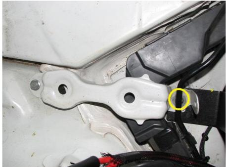
**2.12.** Install AOS with (3) 16mm long BHCS with washers to the bracket as shown. Tighten these bolts to 6-8 ft-lbs max.
