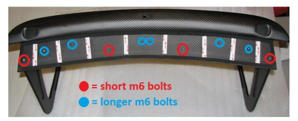
**2.29.** Pull the backing off the double sided tape on the carbon ducktail before install.
