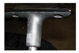
2.3. Remove all the torx bolts on the underside of the OEM wing.
