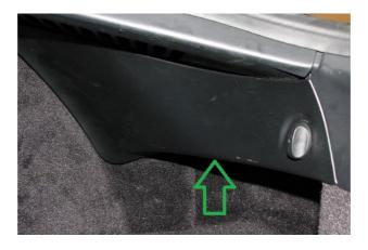
**2.21.** Pull down on the pillar mounts as shown below. They do not need to be fully removed; just pulled down in the rear.
