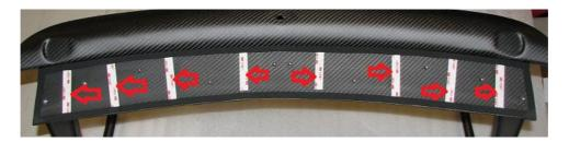
**2.30.** Use care when installing the bolts! Cross-threading bolts into the bungs can cause permanent damage to the duck tail, bung, or both.
