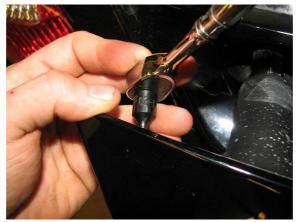
**2.4.** Remove the nut shown below on each side. This will allow the spoiler to be fully removed.
