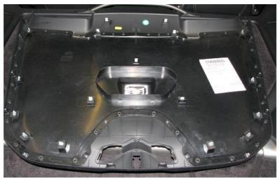
**2.9.** To fully remove the panel the light needs disconnected.
