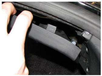
**2.22.** The hatch plastic can now be removed. Pull this forward to remove.
