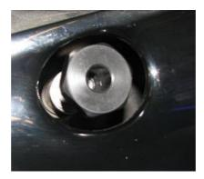
**2.27.** The spoiler mount should be parallel to the rear bumper. Utilize the supplied M8 washers to properly space the spoiler mounts, we found (2) washers worked well for our shop car.
