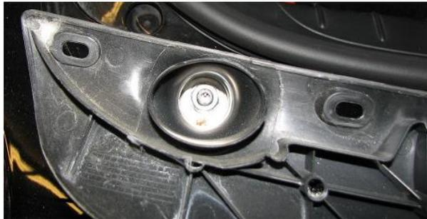
**2.5.** With the spoiler removed, pop the trunk so that we can remove the plastic during drilling.
