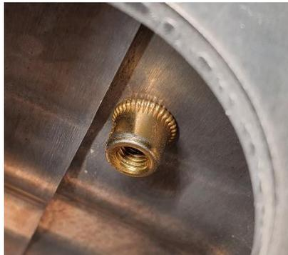
**2.4.** Install the brackets as shown by using two 20mm long M6 BHCS and 18mm washers for the M6 rivet nuts, and 20mm long M8 BHCS with M8 washers for the M8 rivet nuts. A 5mm nylon spacer should be placed between the inner brackets and the sub-frame. Torque the M6 BHCS to 6 ft-lbs, and the M8 BHCS to 12 ft-lbs.
