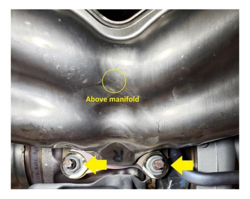
**2.10.3.** From there, remove the three E12 (External Torx) studs, and the small bracket held in with two 10mm bolts.
