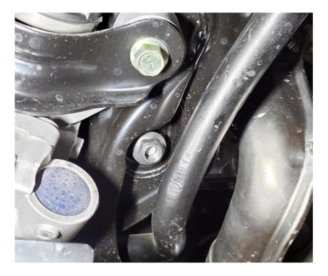
**2.12.** Using a block of wood, jack the engine up by the transmission just behind the bellhousing.
