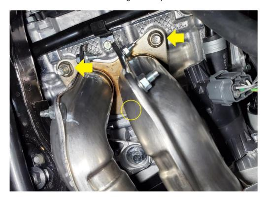
**2.10.2.** Next, remove the three 14mm nuts at the turbo flange connection. You may need a swivel socket / adapter for this.
