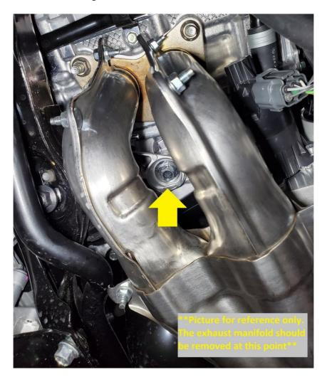
**2.15.** Unbolt the rear motor mount bolt. For this bolt you may need to feel around for it as it is hidden above the crossmember.
