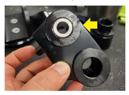
2.4.6. Insert the Bushing Retainer into the Bushing Retainer Bracket. Note: The bushing retainers should be installed so that the locating dowel will be closer to the body work NOT the engine. Use the photo below for reference.
