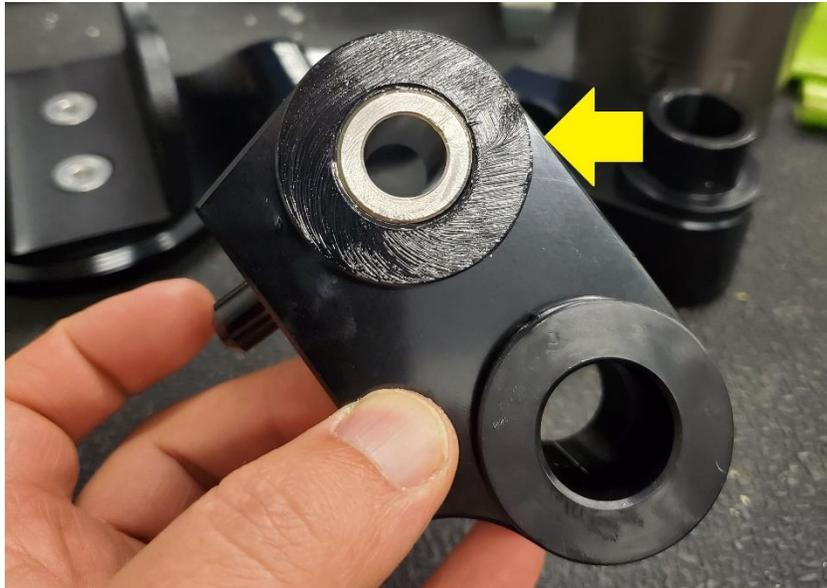
2.4.6. Insert the Bushing Retainer into the Bushing Retainer Bracket. **Note: The bushing retainers should be installed so that the locating dowel will be closer to the body work NOT the engine. Use the photo below for reference.**
