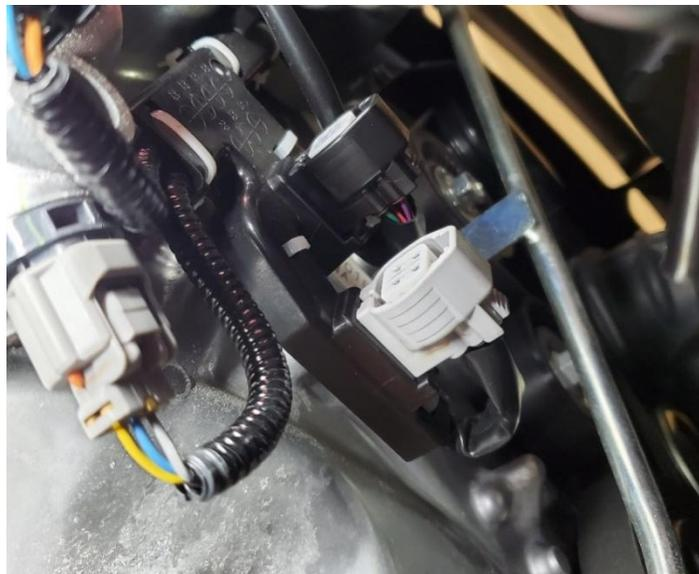
2.8. Unclip the O2 sensor harnesses from the brackets.
