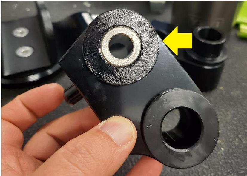
2.4.6. Insert the Bushing Retainer into the Bushing Retainer Bracket. **Note: The bushing retainers should be installed so that the locating dowel will be closer to the outside of the engine bay. Use the photos below for reference.**
