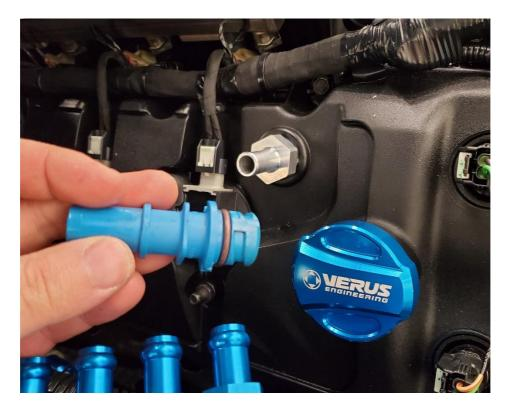
**2.7.** Install the OEM PCV Valve into the Female PCV Valve to 1/2" barb adapter fitting as shown below.
