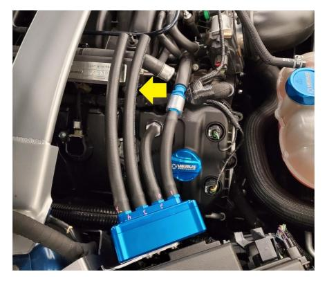
**2.17.** Cut 12 inches of 1/2" hose, and connect it to the AOS as shown.
