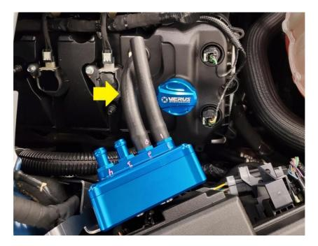
**2.13.** Next, cut 5.25 inches of 1/2" hose, and connect it to the AOS fitting as shown below.
