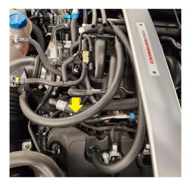
**2.19.** Cut 21.25 inches of 5/8" hose, and insert one of the provided 5/8" -> 1/2" reducers into one end. Connect the other end to the driver side valve cover as shown.
