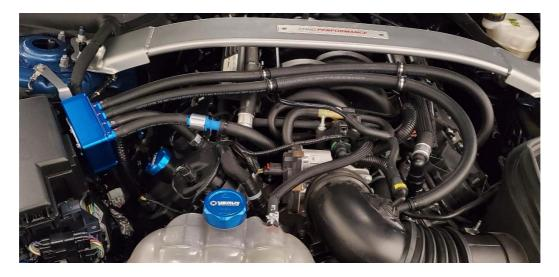
**2.12.** Cut 6.5 inches of 1/2" hose, and connect it to the PCV valve male adapter previously installed on the valve cover and also the AOS fitting shown below.
