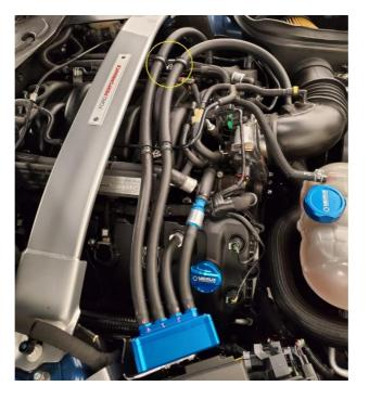
**2.22.** Connect the **11.5**" long 1/2" AOS hose to the **23.75**" long hose going to the intake tube from **2.18**.
