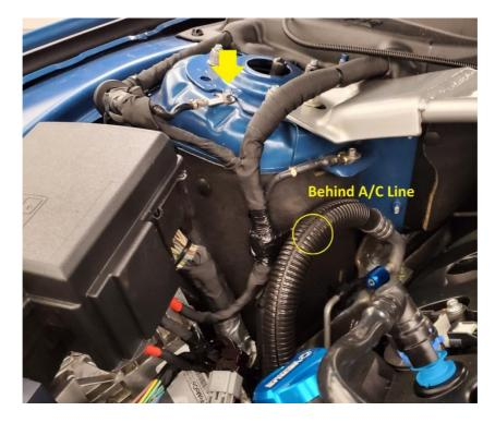
**2.10.** Install the AOS and bracket assembly to the car using the OEM hardware torqued to 6 ftlbs.
