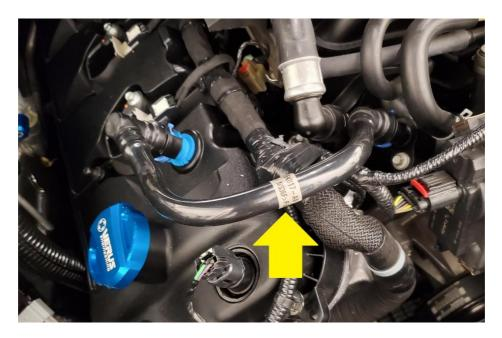
**2.5.** Remove the PCV valve from the passenger side valve cover by turning it counter-clockwise.
