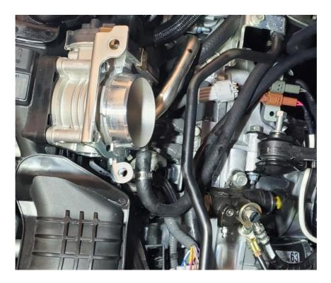
**3.10.** Follow the OEM coolant hose to its' next attachment point behind the driver side cylinder head. Remove the clamp, and the OEM coolant hose all together. Replace that connection with the other AOS coolant hose. Tighten the clamp for the AOS coolant hose.
