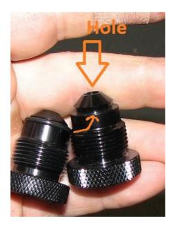
**3.1.** Then, install the black 6AN to 1/2" barb into this and torque to 8 ft-lbs. A photo of this is shown below. When installing the black 6AN to 1/2" nipple, do so with the knurled fitting already installed on the AOS.
