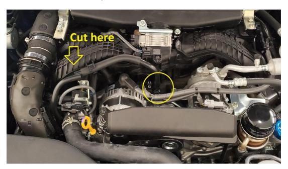
**2.18.** Where the tube meets the fitting for the engine breather tube slice the tube lightly where it is pressed onto the fitting. We recommend doing multiple light slices to prevent damaging the fitting. Once you slice through the tube, remove it.
