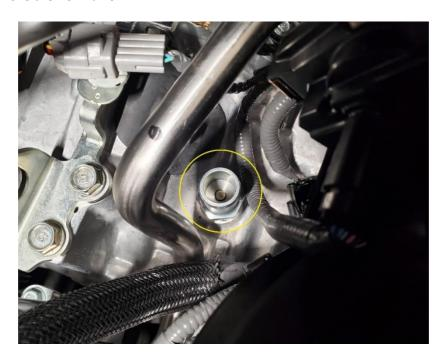
**2.8.** Replace the PCV valve in the engine block with the provided NPT to 1/2" barb fitting. Clean and degrease the threads on both the fitting and the engine block (make sure no debris falls into the engine), and apply thread sealant to the threads on the provided fitting. Tighten the fitting about a 1/4 turn past snug. These are tapered threads, and should **NOT** be bottomed out.
