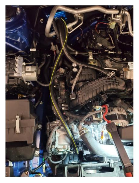
**2.21.** Next, cut 35" of 1/2" hose, and route it from the last AOS fitting available to the metal engine breather tube. Route this next to the hose going to the turbo inlet, and then cross under the intake manifold.
