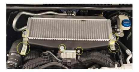
**2.3.1.** Disengage the retaining ring on the charge pipe. Do this by pulling up on the retaining ring. It is seated in the disengaged position in the below images.
