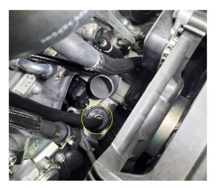
**2.18.2.** With the metal clip released, pull the tube out and perform the same steps to remove the tube from the fitting.
