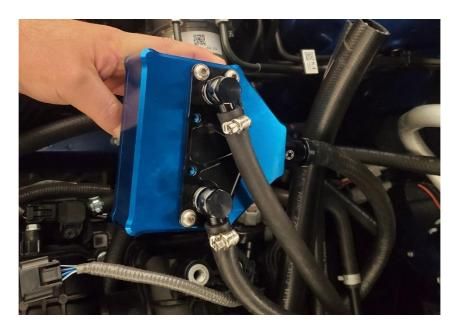
**3.6.** Bolt the AOS to the fire wall with the two M6 serrated flange nuts just as you would have in **2.5**. Torque the nuts to 6 ft-lbs.
