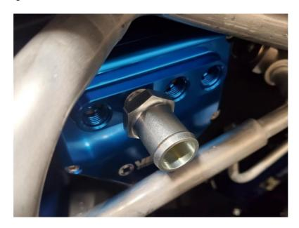
**2.10.** With the PCV valve installed, we now need to install the rest of the 1/2" barb fittings to the AOS. Thread them hand tight, making sure they are bottomed out and the o-ring is fully engaged.
