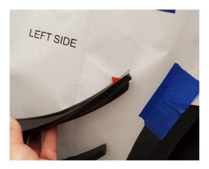
**2.10.** Once you're happy that the placement of the dive plane is correct, begin pulling the red backing off while holding the dive plane in place.
