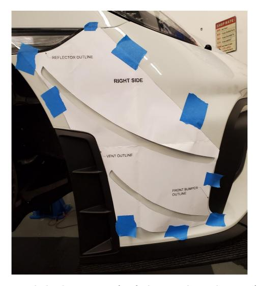
**2.6.** Prepare the dive plane mounting surfaces for the VHB tape by using the same 50 / 50 Isopropyl alcohol / water solution, and a clean microfiber towel to clean them thoroughly.
