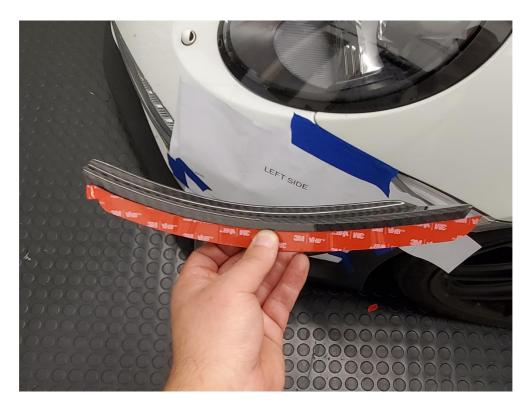
**2.8.** For the install, the slightly larger units are the top dive planes, while the slightly smaller units are the bottom dive planes.
