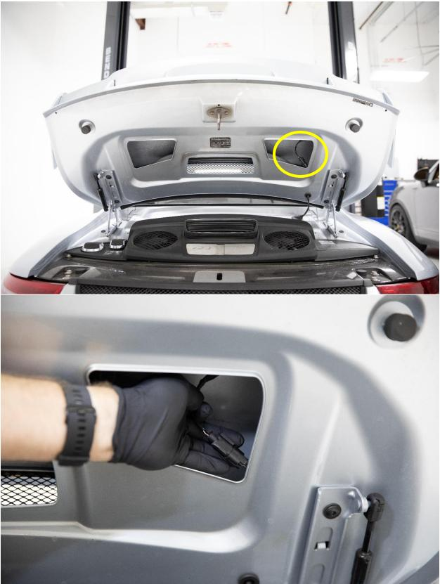
**Step 1:** Open the trunk and disconnect the 3<sup>rd</sup> brake light cable.
