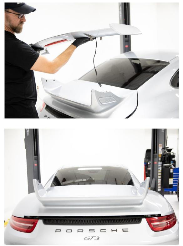
**Step 4:** Install the wing risers. Use a microfiber to clean the surface. Use a 5mm HEX to install the new hardware provided. **NOTE:** Leave the hardware slightly loose. **Do not tighten the bolts down all the way!**
