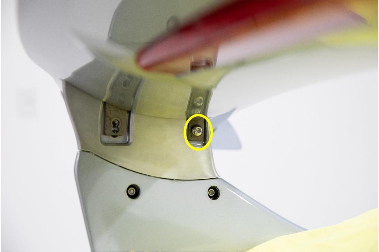
**Step 7:** Adjust the spoiler to your desired height. Make sure to properly align each side of the spoiler.
