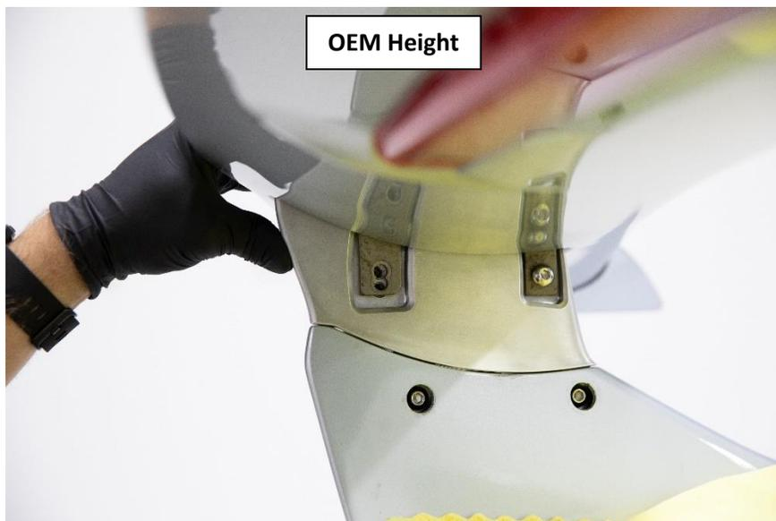
**Finish:** Make sure to tighten all hardware and re-connect the 3<sup>rd</sup> taillight brake cable.
