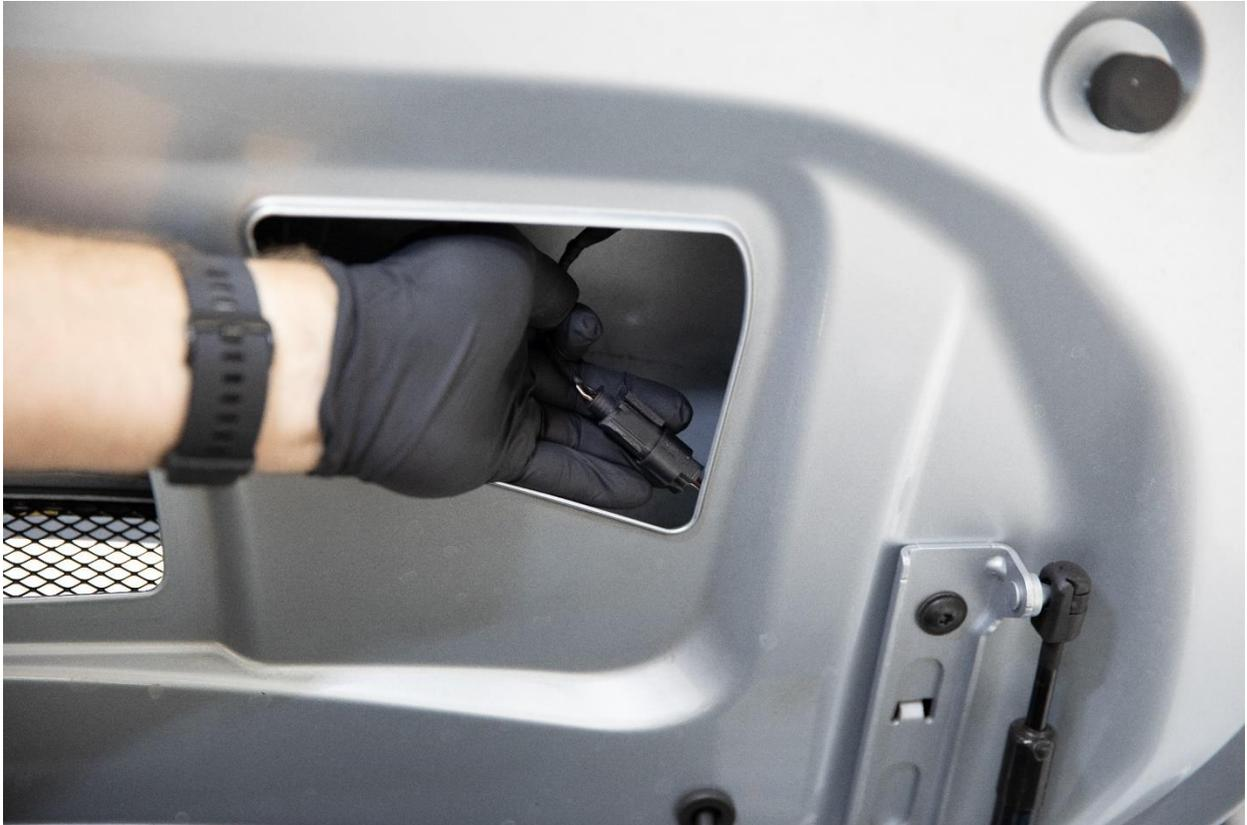
**Step 2:** Remove the four (4) rubber gromets on the inside of the spoiler. You can use a plastic pick to remove the gromets. Be careful not to damage the paint. Then, remove the hardware holding the spoiler in place using a T40 socket.
