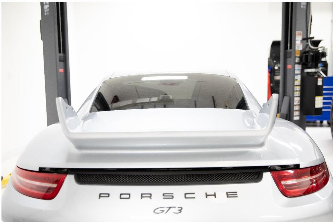
**Step 4:** Install the wing risers. Use a microfiber to clean the surface. Use a 5mm HEX to install the new hardware provided. **NOTE:** Leave the hardware slightly loose. **Do not tighten the bolts down all the way!**
