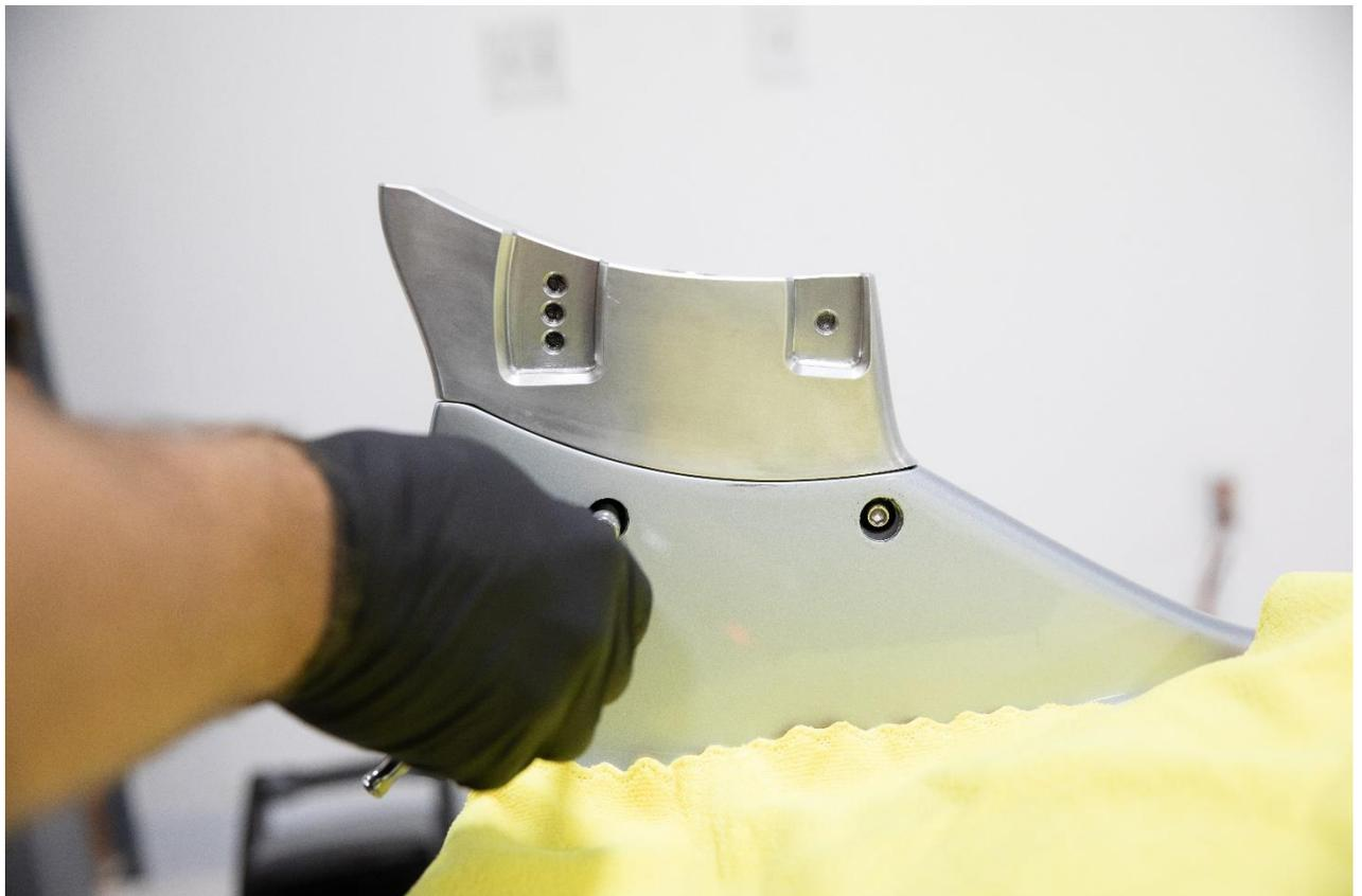
**Step 5:** Place the wing on the risers. Make sure to feed the brake light cable all the way through so the spoiler can seat properly.
