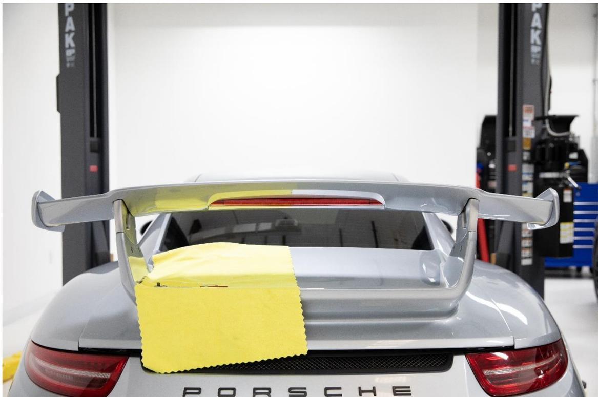
**Step 6:** Using the 5mm HEX, install the hardware on the front of the spoiler first. **NOTE:** Leave the hardware slightly loose. **Do not tighten the bolts down all the way!**
