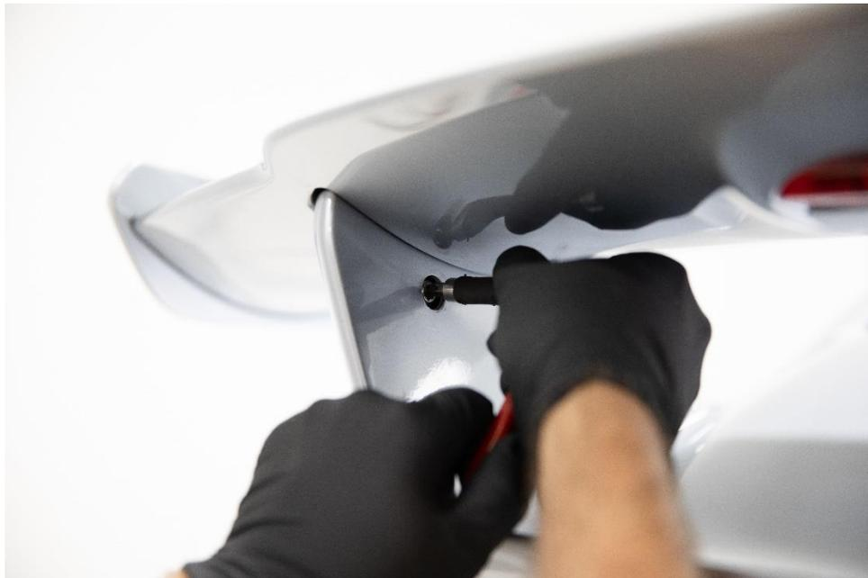
**Step 3:** Carefully remove the spoiler. Make sure the brake light cable is clear from being caught inside the spoiler.
