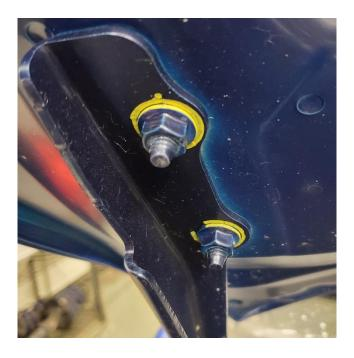
2.17. Install the hood louvers into the hood verifying that the studs all line up into the holes, and that it sits flush on the hood. Using the supplied 11/32" serrated flange nuts start all the nuts first, except for the front three studs. For the front three studs, first install the supplied wicker as shown, then start the nuts. The wickers are directional.
