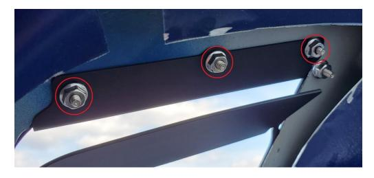
**2.18.** When all nuts are <u>finger tight</u>, use the 11/32" socket to add approximately 1/8 turn to each of the nuts. Watch the top of the hood louver to ensure you are not pulling the stud down through the material. **MAXIMUM TORQUE IS 17 IN.LBS!** The nuts are serrated and resist backing off, they do not need significant torque.
