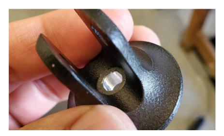
**2.19.** Using two low profile 25mm long SHCS, slide them through the top of the clevises and thread them into the rivet nuts just installed. Orient them parallel with the front of the car as shown, and torque to 6 ft-lbs.
