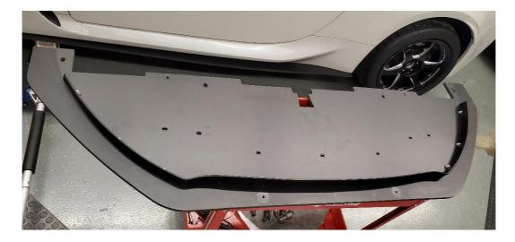
**3.14.** Before installing the splitter on the car, install the supplied rubber edge seal on the top side of the air dam to prevent the air dam from digging into the bumper or paint when installing. This rubber seal also helps seal the air dam with the factory front fascia when it is installed.
