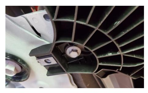
**2.8.** Finally, remove the bumper cover support brace by removing the two clips holding it in from the top.
