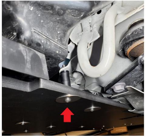
**2.30.** Finally, use two 40mm BHCS, fender washers, 5mm nylon spacer, 18mm washer, and M6 serrated flange nut to bolt the splitter to the last outer hole on the bumper ( closest to the wheel well). You will need to push the fender liner to the side to get the nut and washer above the bumper as shown. **BRZ Install Note:** BRZ models do not have pre-drilled holes in
