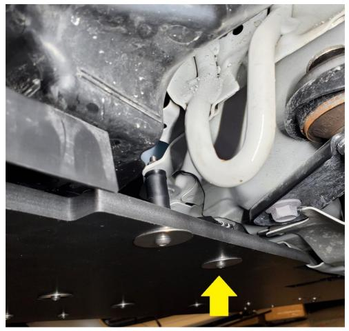
**2.29.** Then, using the 60mm BHCS, fender washer, two 15mm nylon spacers, one 5mm nylon spacer, and M6 serrated flange nut to bolt the splitter to the lower radiator support. Do this on both sides. This is shown below.
