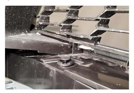
**2.9.** Install five M6 Plastic rivet nuts into the bumper cover support brace. Use the holes that the push clips came out of (The holes can be identified by a "star" shaped pattern surrounding them). Open the holes up with a 3/8" drill bit if needed. Make sure you install the rivet nuts on the correct side. You should be installing them into the side shown below.
