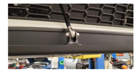
**2.28.** Use two 45mm long BHCS, fender washers, 15mm, and 5mm nylon spacers to bolt the splitter to the radiator support splash shield on both sides (the plastic cover with the metal U-nut). This is shown below.
