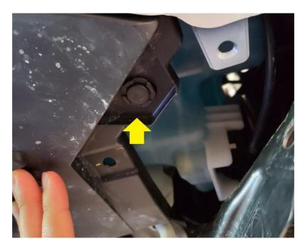
**2.7.** With the splash guard removed, we can now remove the lower radiator support splash shield. Most of the hardware holding this part in should have been removed in **2.4**. All that Confidential: Property of Verus Engineering. Not for Distribution outside intended recipient list.
