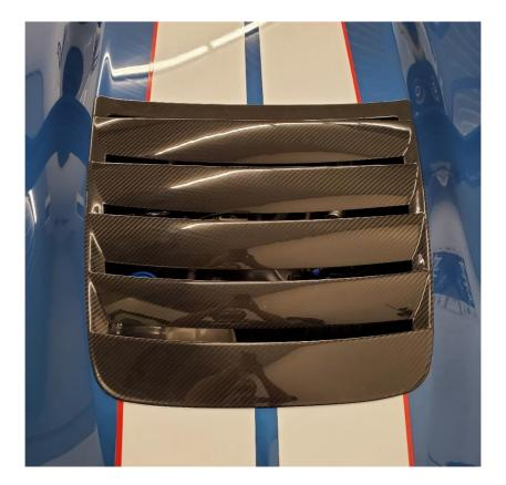
**2.17.** Reinstall the hood if you haven't already, and reassemble the washer system in reverse order. Be sure to confirm that the hood alignment is correct before attempting to shut it. If you marked the nuts in **2.6**, you shouldn't need to do any further adjustments. However, in the event you need to make adjustments, simply loosen the 13mm nuts to move the hood in the desired direction.
