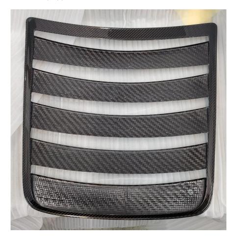
**2.14.** Apply the pre-cut 3M VHB tape to the bottom side of the Carbon Hood Vent. Preferably have the red backing facing up.
