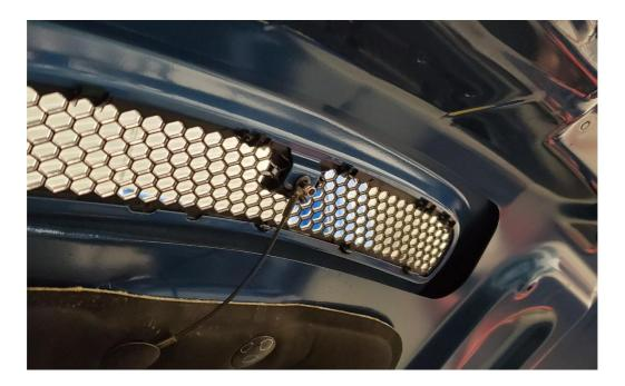
**2.5.** To disconnect the washer nozzle hoses, spread the black plastic ring.
