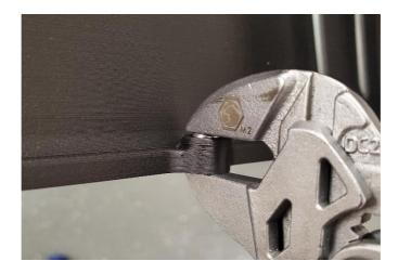
**2.8.** Using the opposite side endplate, temporarily bolt it up upside down using two 20mm long M4 FHCS (Flat Head Cap Screw).
