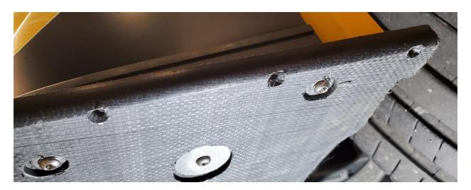
**2.11.** We recommend deburring the holes by simply using a sharp razor blade to cut off the "hairs" that may remain.
