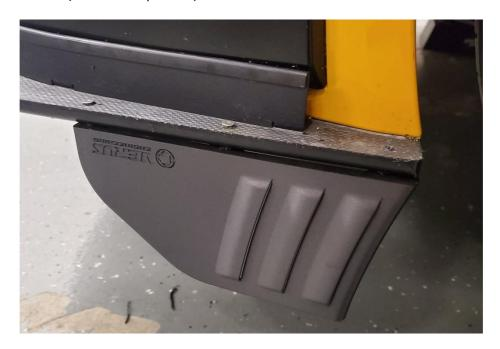
**2.9.** Mark the last hole from the bottom of the splitter, and drill to 5/32".
