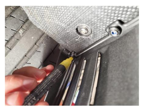
**2.10.** Counter the three holes on the **BOTTOM** side of the splitter.
