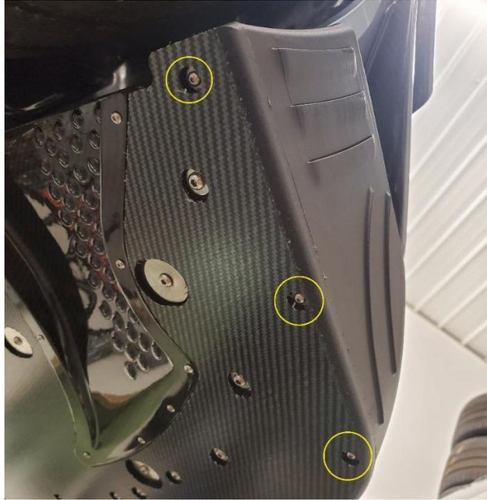
**2.4.** Press the M4 Nyloc nuts into the endplates as shown. Using a pair of pliers will help.
