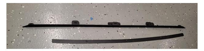
**2.50.** The flat bracket with the three pressed on nuts will go above the bumper lip, and the bent bracket will go below the bumper lip. These two brackets should sandwich the bumper lip as shown. Use three 16mm long M6x1.0 BHCS, and torque to 6 ft-lbs. These bolts should line up with the holes for the push clips removed in **2.10**. **991.2 owners will use three 12mm long M4 BHCS instead. Torque these to 4 ft-lbs.**
