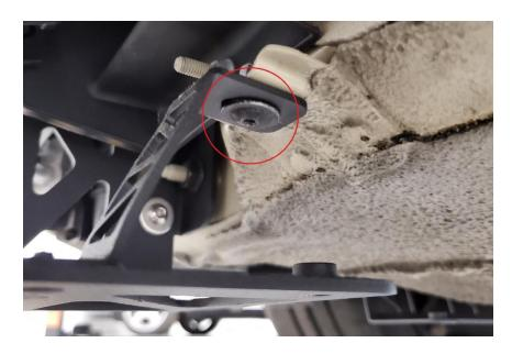
**2.29.** Install both rear outer brackets. Remove the OEM bolt that attaches the air dam, and reuse the bolt and hole to install the bracket as shown. The passenger side is pictured.
