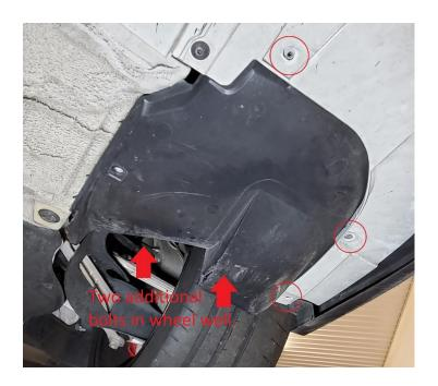
**2.11.** Remove the front center splash guard with a T25, and clip removal tool for the three push clips. This will not be re-installed.
