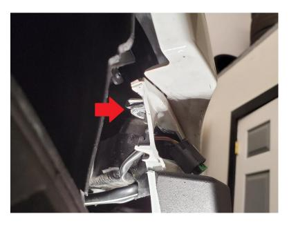
**2.15.** On both sides, disconnect the connector behind the fender liner. If you peel the liner back, the connector is about 12 inches inboard. You can also follow the harness coming from the marker light area t.
