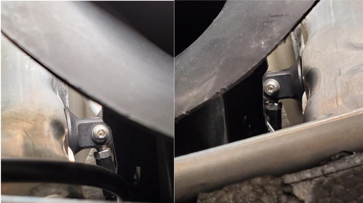
**2.38.** Using the same method and hardware, install the splitter ties to the cross-brace clevises.
