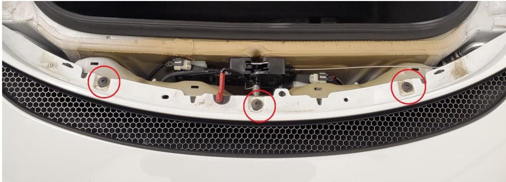
2.7. Using a small hook pull out the bumper release tabs on the inside of the headlight housing.
