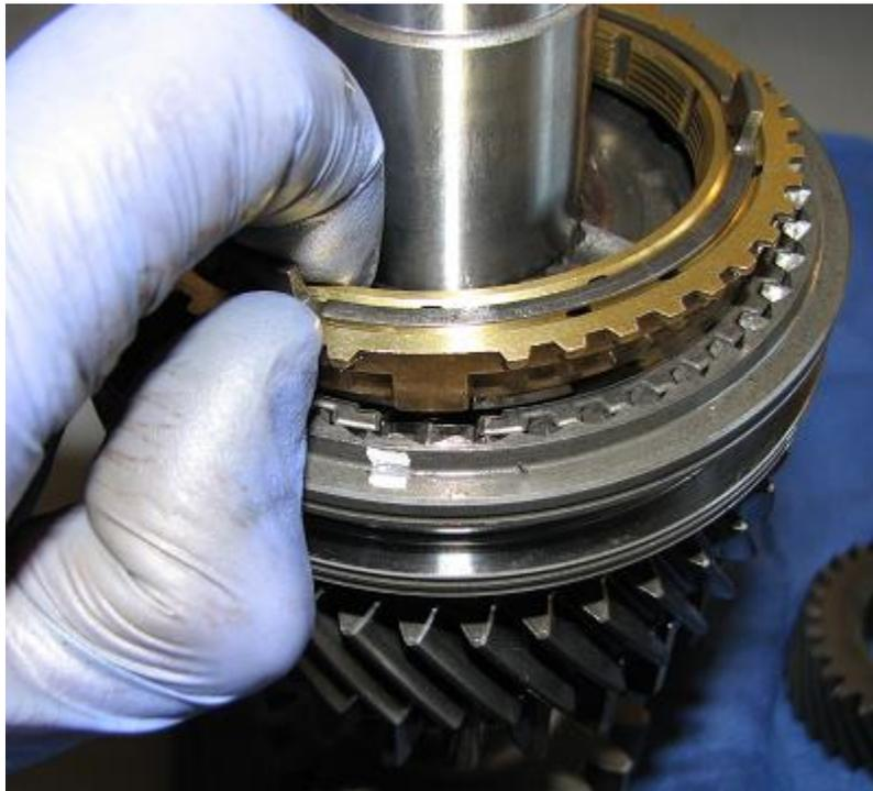
29) Install the 1<sup>st</sup> gear's shift restrict ball as shown below.
