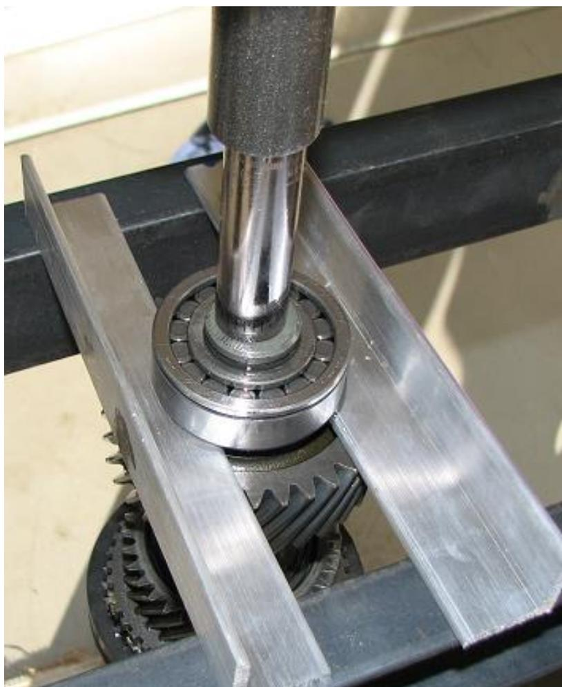
5) Remove counter drive gear's snap ring located below this bearing.
