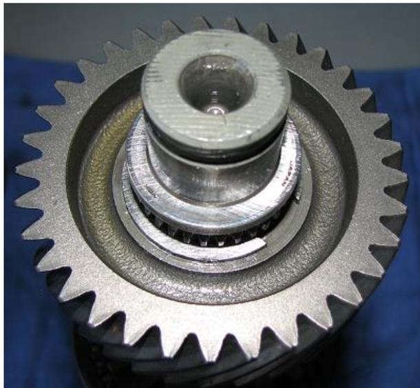
17) Install front counter gear bearing as shown below. The snap ring groove points upward.
