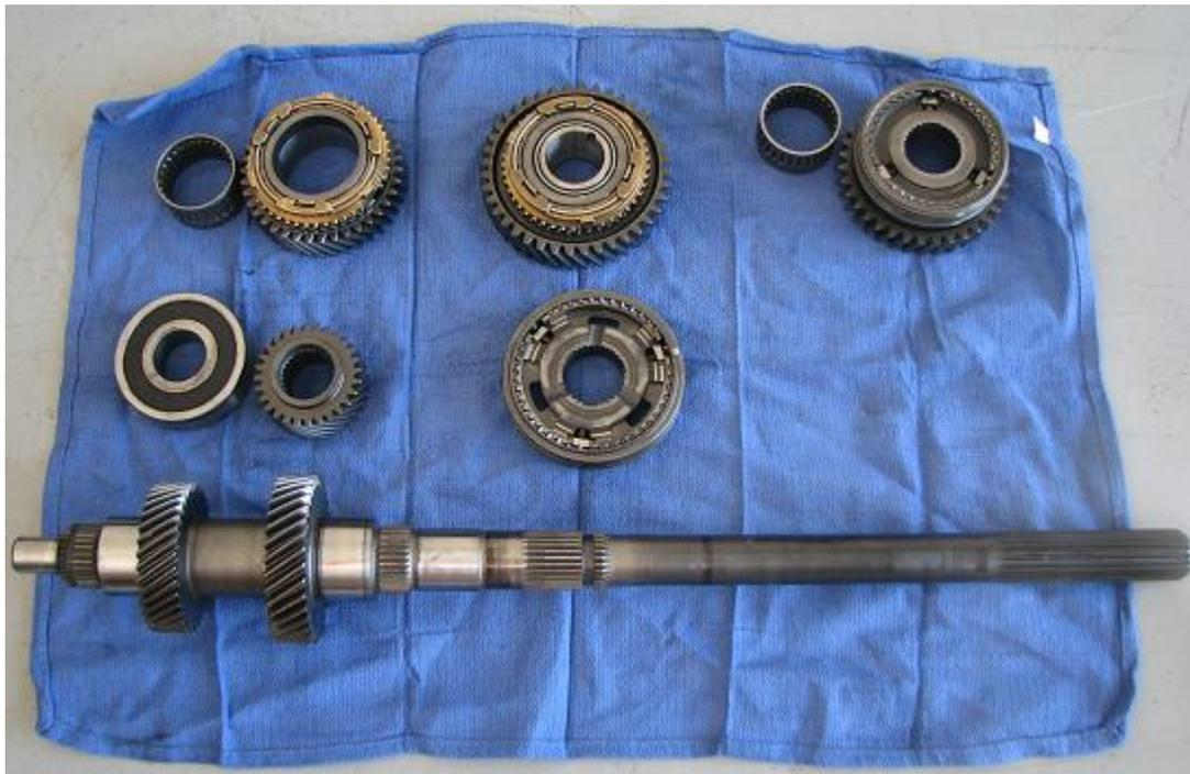
26) Time for re-install on the billet output shaft. Place 2<sup>nd</sup> gear's needle bearing (oiled) on the shaft, slide 2<sup>nd</sup> gear down on the shaft, 2<sup>nd</sup> gear synchro, and then the 1<sup>st</sup>/2<sup>nd</sup> gear shift/clutch hub. This requires a long special service tool as shown below.
