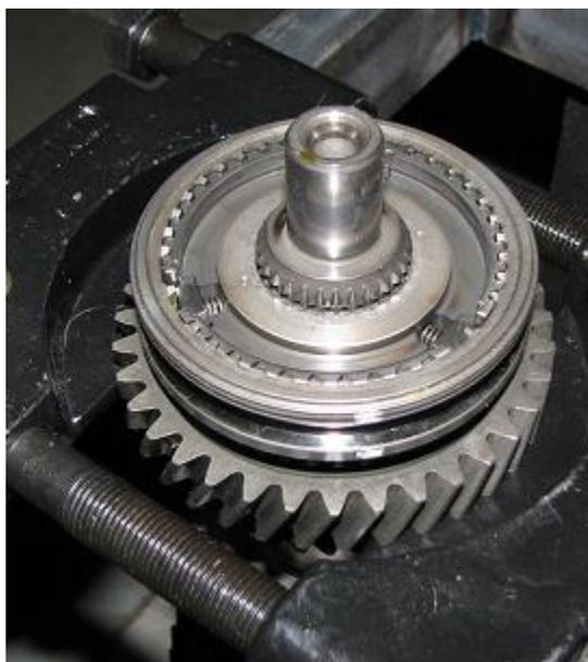
21) Remove 6<sup>th</sup> gear's snap ring, shown below, with two screw drivers and a hammer.
