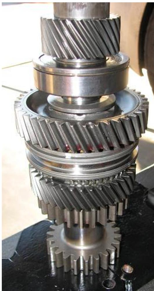
32) Install the snap ring on the end of 6<sup>th</sup> gear.
