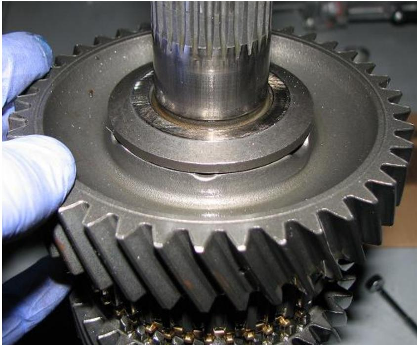
31) Install the output bearing and 6<sup>th</sup> gear by pressing them on.
