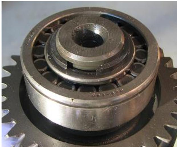
19) Remove 5<sup>th</sup> / reverse gear's clutch/shift hub assembly's snap ring via snap ring pliers.
