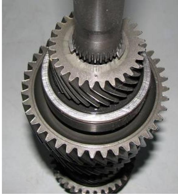
22) We remove 6<sup>th</sup> gear, output bearing, and 1<sup>st</sup> gear in one step. This requires a bit more force but all three can come off at the same time.
