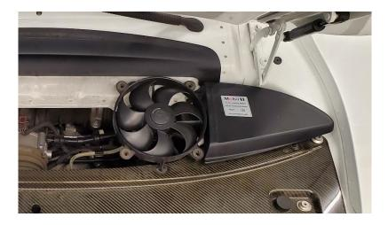
**2.12.** Disconnect the connector below this cover plate. **NOTE: Until this connector is plugged** back in, do not shut the trunk. This connector is shown below.
