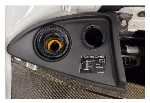
**2.9.** Remove the coolant and oil fill port cover plate. Do this by removing the 10mm head bolt, and releasing the hose clamp that attaches the oil filler port to the filler neck.
