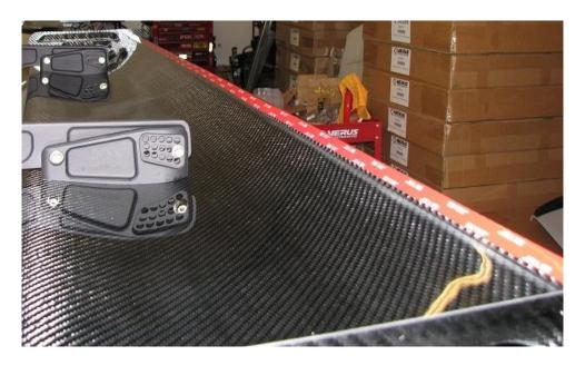
**2.31.** Clean the gurney flap on the surface to be installed on the rear wing.
