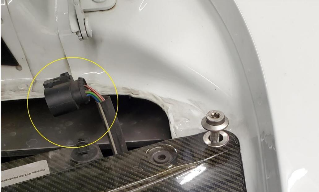
**2.13.** Now we need to remove the carbon panel that houses the trunk latch.
