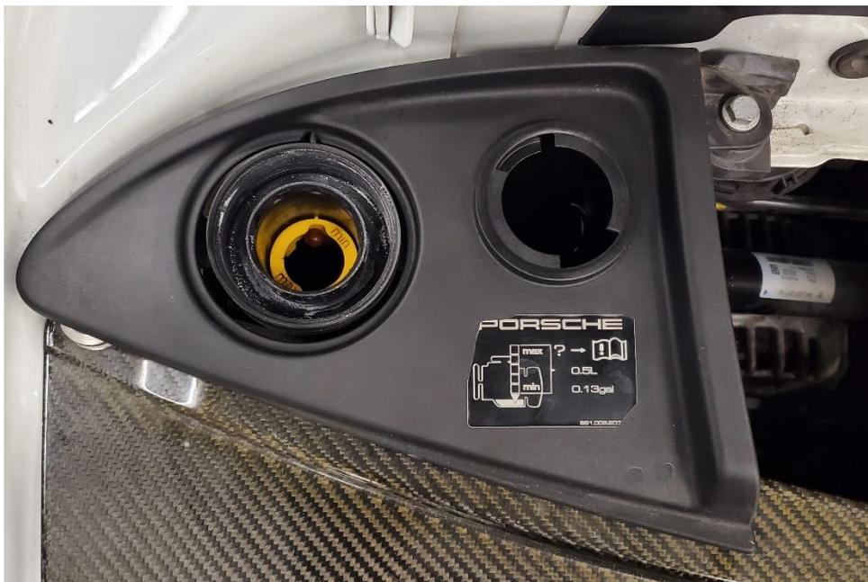
2.9. Remove the coolant and oil fill port cover plate. Do this by removing the 10mm head bolt, and releasing the hose clamp that attaches the oil filler port to the filler neck.
