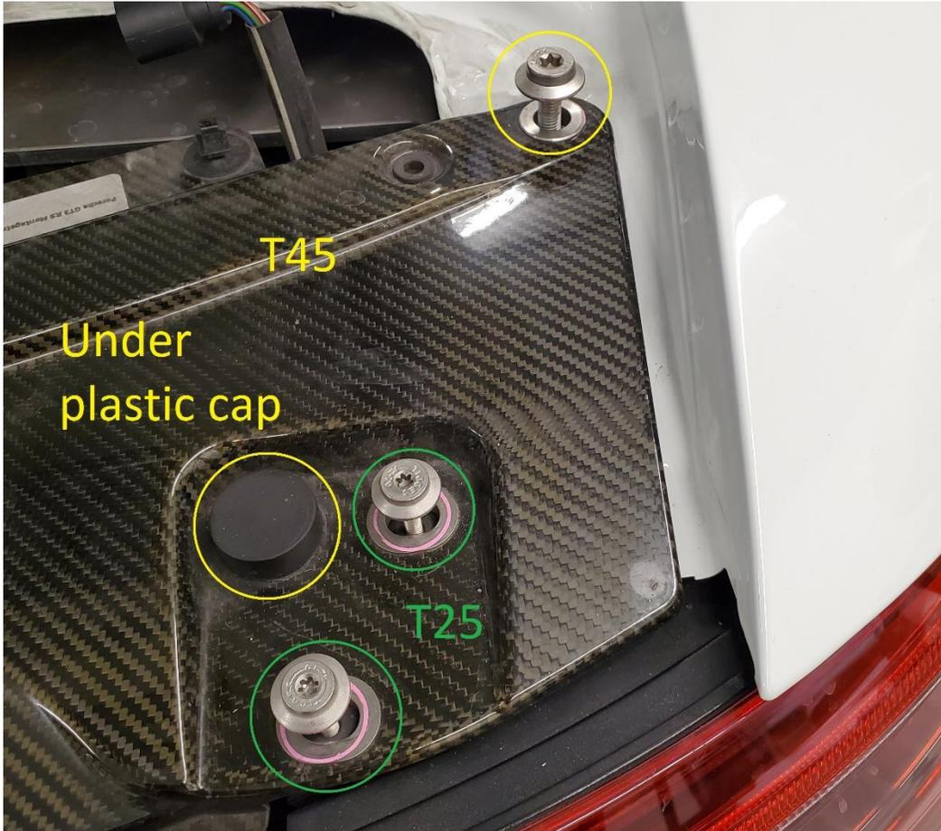
2.16. Remove the T30 bolts attached to the bumper.
