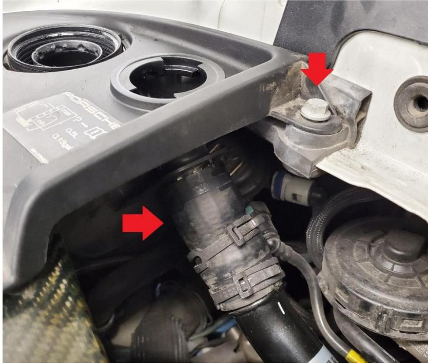
**2.10.** Once the bolt and the clamp are removed, and released pull up on the cover plate to release the rubber grommets. Also disconnect the oil filler neck hose. **NOTE: It is a good idea to clean around these two filler ports prior to removal as road grime and debris may fall into either port.**
