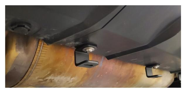
**2.14.** Loosely install both side brackets / strakes using six 20mm BHCS, and washers. These pieces should slide up, and down to aid in setting the correct height for the final installation.
