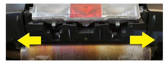
**2.9.** Install three plastic M6 rivet nuts into the holes shown below. Follow the diagram for instructions on how to use the rivet nut installation tool. The holes should already be a suitable size however, if needed, use the 3/8" drill bit to open them up.
