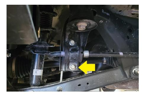
2.6. Install the bracket between the sway bar mount, and the sub-frame. Use the lower bolt. You may fully tighten these bolts at this time. Make sure the bracket is level with the ground. Torque the bolts 22 ft-lbs. NOTE: BRZ's will still mount the bracket in the same manner. The bracket will just be in a different spot due to the difference in the OEM sway bar mount. Both are pictured below.
