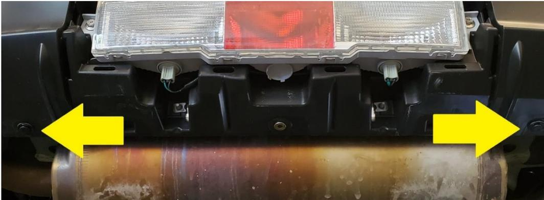
2.9. Install three plastic M6 rivet nuts into the holes shown below. Follow the diagram for instructions on how to use the rivet nut installation tool. The holes should already be a suitable size however, if needed, use the 3/8" drill bit to open them up.
