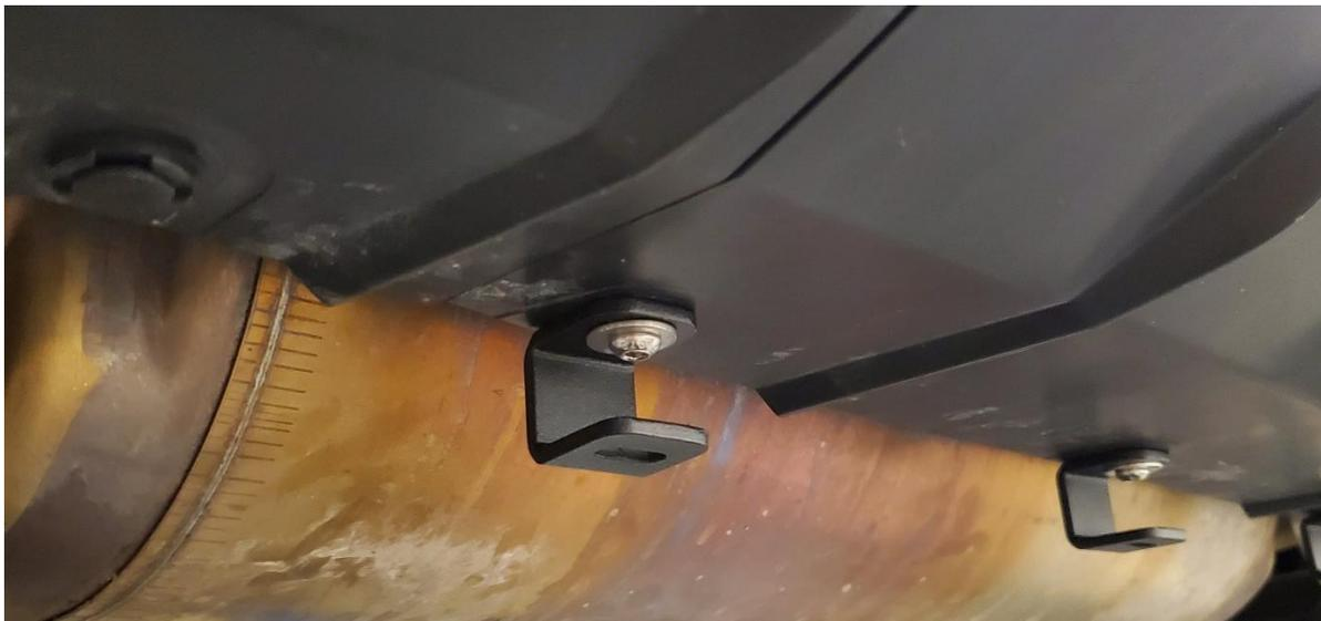
**2.14.** Loosely install both side brackets / strakes using six 20mm BHCS, and washers. These pieces should slide up, and down to aid in setting the correct height for the final installation.
