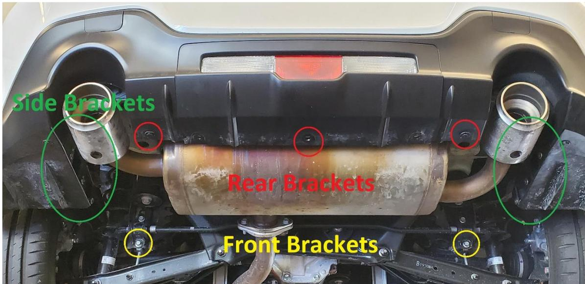
2.4. First, we will start with the front brackets mounted to the sway bar mount.
