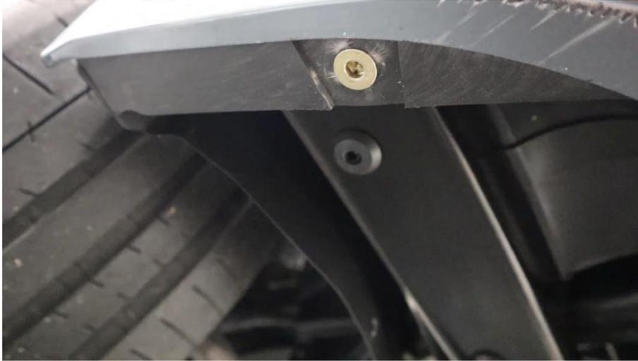
**3.15.** Below is a photo of a properly installed rivet nut.
