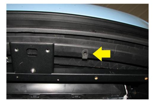
**2.14.** Assemble the Splitter halves by lining up the "zipper" pieces and tapping them together with a soft faced hammer. Once they are interlocked, use an M4x.7 BHCS, M4 fender washer, M4 small diameter washer, and nyloc nut to complete the assembly. Torque to 4 ft-lbs. The nyloc nut and fender washer should be on the top side of the splitter.
