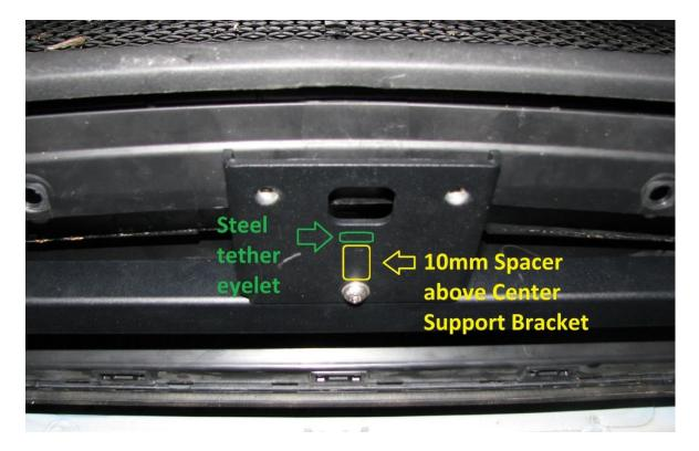
**2.13.** Install four M6 U-Nuts into the bumper mounting holes as shown below.
