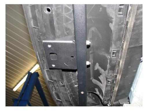
**2.9.** From there, bolt the Cross Brace assembly to the Main Splitter Brackets as shown, use four 16mm BHCS, and 18mm washers. Torque to 6ft-lbs. Make sure the bumper slides in the slots at the ends of the brace.
