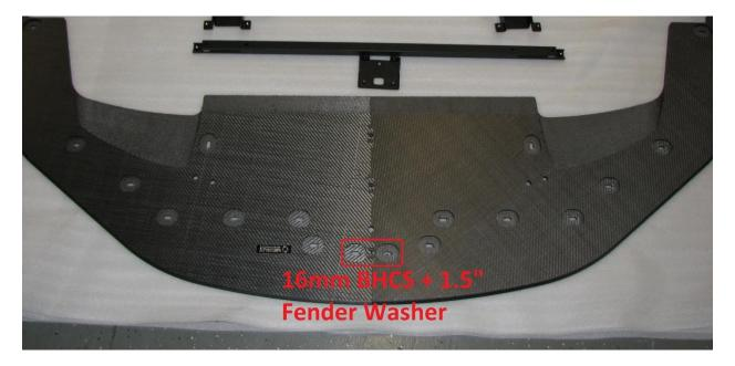
**2.19.** Install two one inch long #10 THCS with the #10 washers into the rearmost outer bolt holes. These should thread into OEM mounting locations.
