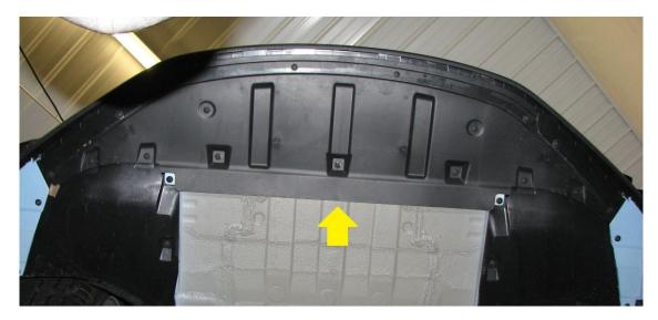
**2.4.** Remove the front splash shield. Several T30, and T25 bolts hold it on.
