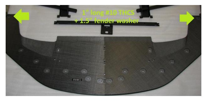
**2.20.** Install 20mm long BHCS with 1.5" fender washers into all remaining holes.
