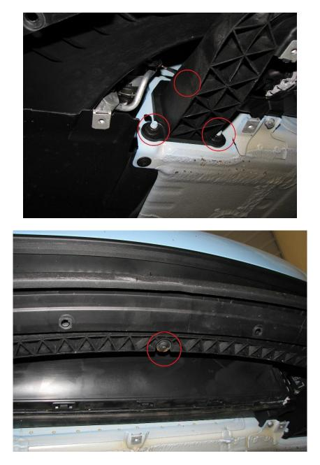
2.6. Bolt the Main Splitter Brackets to the chassis using the 13mm nuts for the pedestrian bar. Torque to 15ft-lbs. These brackets are mirrored, so be sure to mount them to the correct side. When bolted up, they should allow the outer bracket tubes to be installed so that they point rearward. Refer to the image in 2.2 for a visual aid
