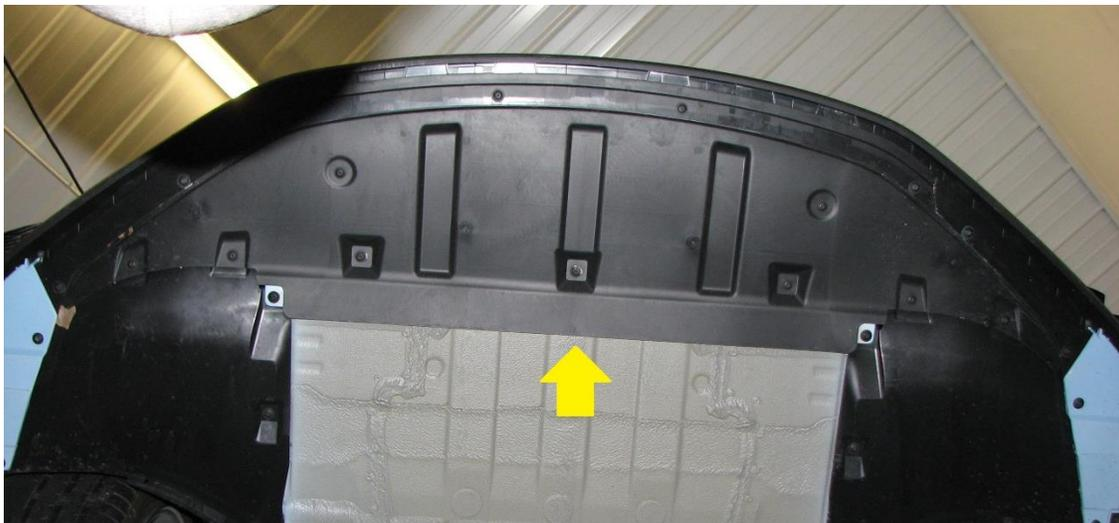
2.5. This will expose the pedestrian bar. Remove the six 13mm nuts holding it to the chassis, and the T30 bolt that attaches to the steel tether.
