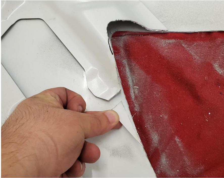
**2.13.** Before we begin final installation of the hood vent, place it on the hood, and make sure you cannot see any of the under-hood structure through the vent. If you can, trim it back until it is no longer visible.
