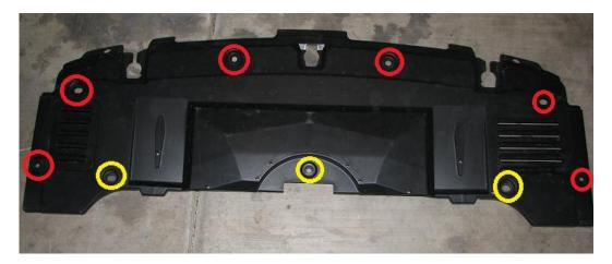
**6.3.** Now comes the hardest part of the install, installing the rivet nuts. Please view the next photo to ensure you are installing them in the correct holes. No holes should be drilled!!! This photo shows only the passenger side of the car, the driver's side is a mirror image of this.
