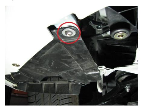
**6.7.** Install the splitter with the remaining M6x1.0 x 25mm BHCS with washers on each of the rivet-nuts. Utilize the aluminum spacer and the 30mm long BHCS on the two most rearward holes. We suggest to leave all bolts loose until they are all in and then tighten from the inside out. We also suggest you have the splitter held up by 4 or more bolts before letting the splitter free hang.
