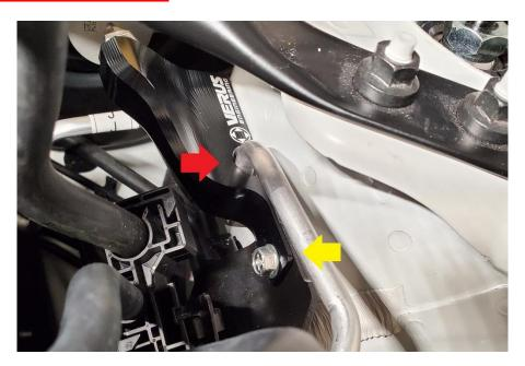
**2.8.** Next, install the 12mm long M6 SHCS into the counter-bore as shown. Torque to 6 ft-lbs. Also torque the previously installed 10mm head bolt to 6 ft-lbs.
