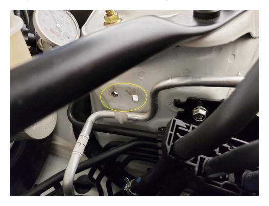
**2.6.** Remove the 10mm head bolt holding the fuel line bracket.
