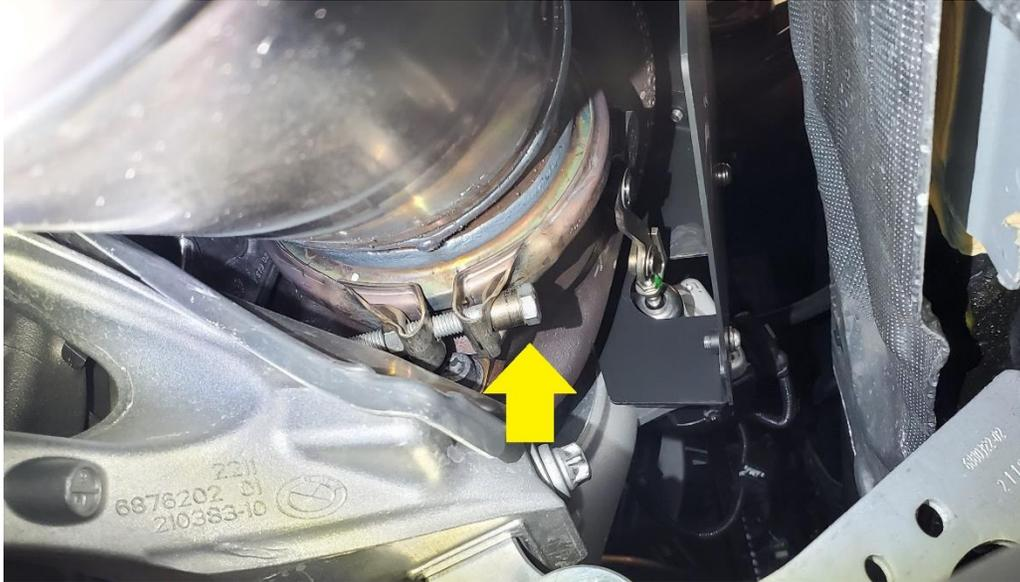
**2.6.2.** Remove two 13mm downpipe bracket nuts.
