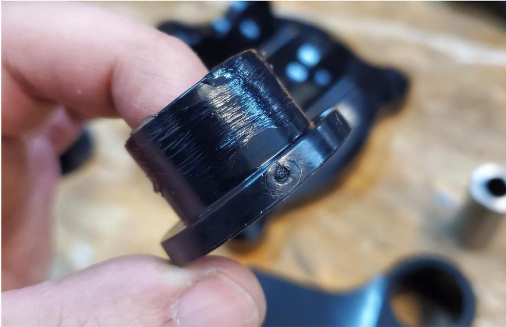
**2.12.3.** Press the bushings into the bushing retainer followed by the bolt sleeve.
