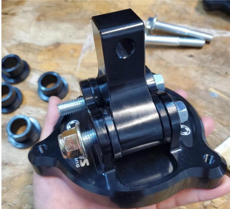
**2.12.5.** Install the engine mount and engine mount bracket in the reverse order. Start all bolts first. Torque the E12 bolts to 28 ft-lbs.
