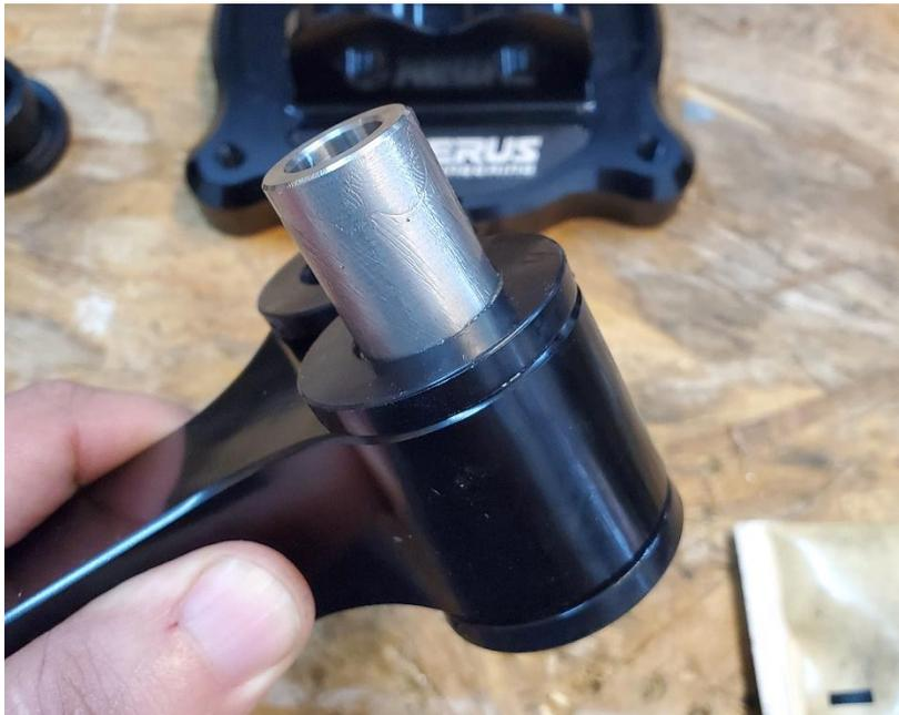
**2.12.4.** Push the bushing retainer into the base, and assemble the engine mount using the M12 bolts and nyloc nuts. Torque to 60 ft-lbs. Note: a dab of Loctite for extra security does not hurt either.
