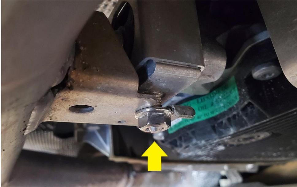
**2.6.4.** Loosen the rear exhaust clamp connection for the downpipe.
