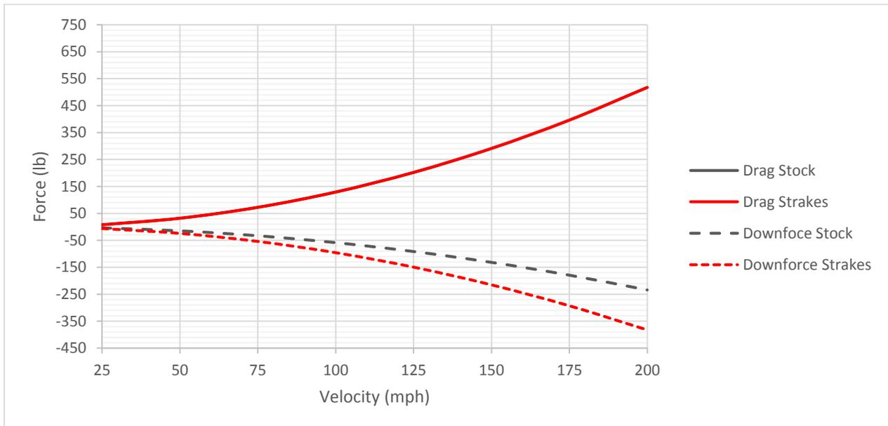
Figure 1.2.1: Aerodynamic Forces at Speed
