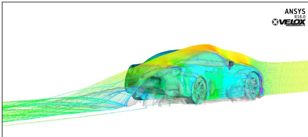
Figure 1.3.5: Streamlines and Transparent Q-Criterion
