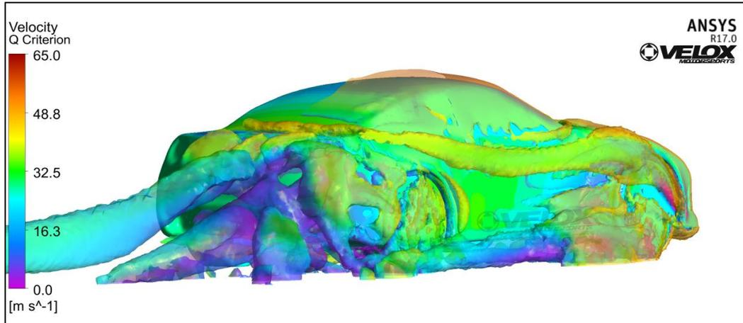
Figure 1.3.4: Q-Criterion (vorticity) with Velocity Plot
