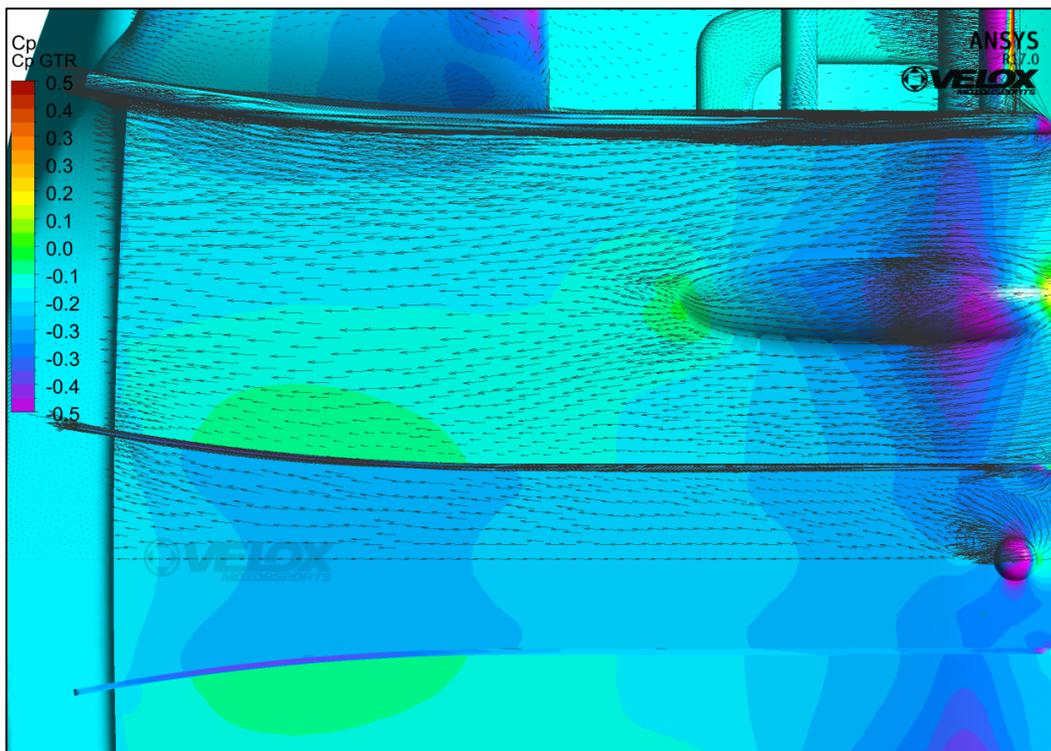
Figure 1.3.3: Diffuser Surface Cp (Coefficient of Pressure) with Surface Vectors
