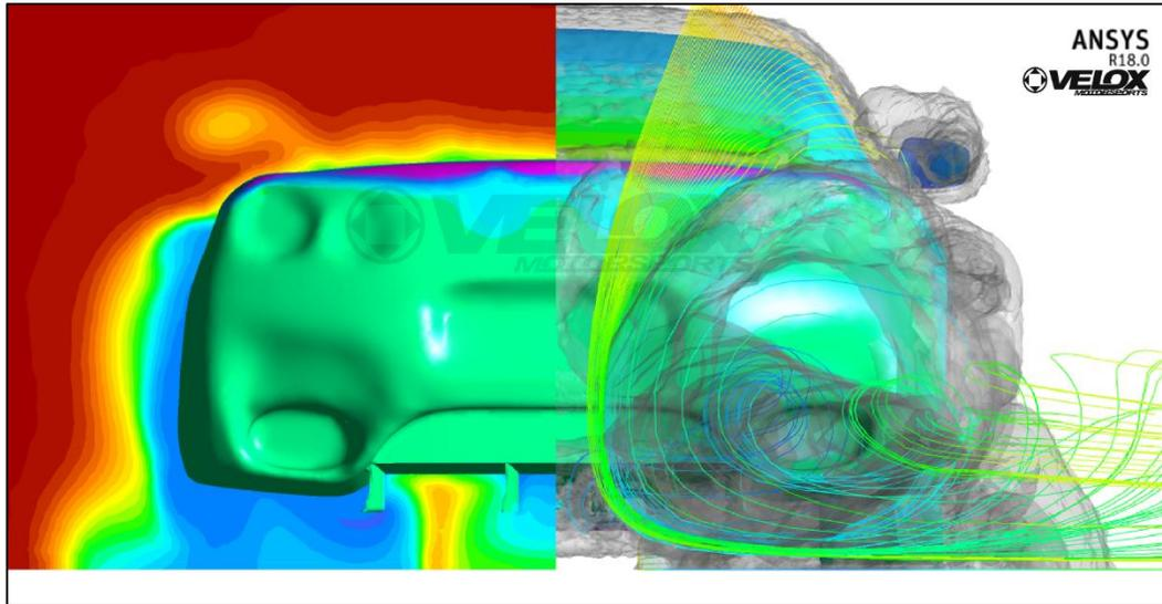
Figure 1.3.6: CpT Cut Plane Behind Rear Tire
