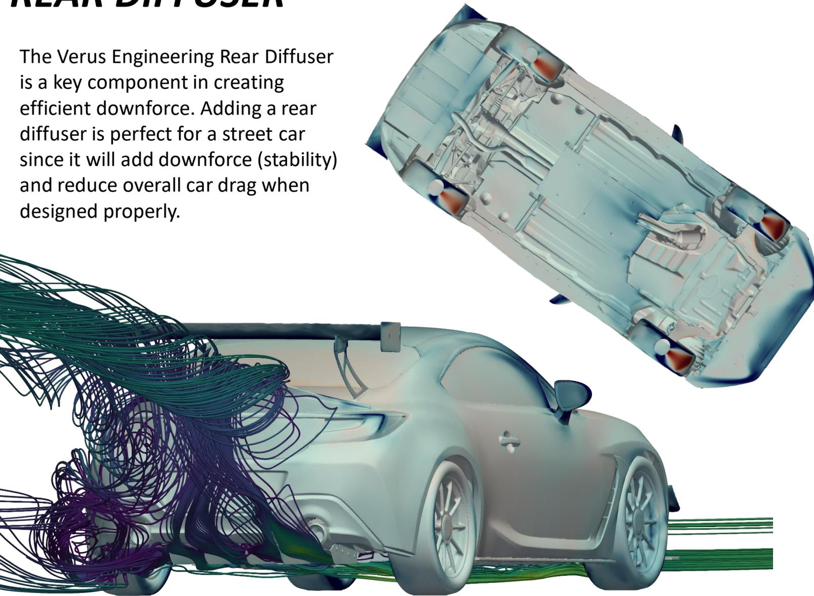
A large portion of the drag on a normal road vehicle, like the GR86 Platform, is from pressure drag. Pressure drag is caused by the low pressure region behind the vehicle which wants to pull the car rearward. This low pressure region behind the vehicle is called the wake region.
