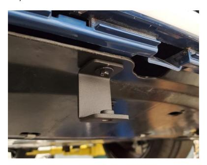
**2.24.** Now that all the brackets are installed, we will want to level them so that they are the same height. Loosen the four bracket bolts pictured below in order to slide the bracket up or down as needed.
