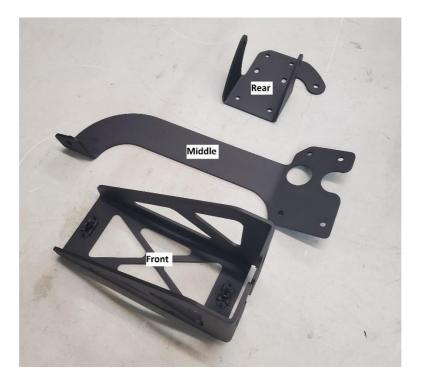
**2.21.2.** Using eight 25mm M6x1.0 BHCS, 18mm washers, and M6 serrated flange nuts, bolt the three pieces together in the orientation shown below. Use the top two holes and the bottom two holes. The center holes are for installing to the car. Driver, and passenger sides will be mirrors of each other. They should also line up with the holes in the splitter.
