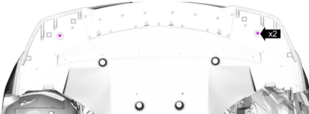
**2.3.3.** Finally, remove the fender liner clips (on both sides) to peel back the fender liner enough to remove the retaining clips for the front lip.
