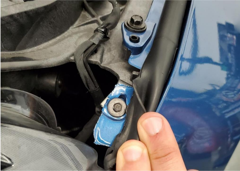
2.7. Remove the wheel well clips to gain access to the corner bolts. You will only need to remove enough to peel the liner back. You may also completely remove the liner if you like.
