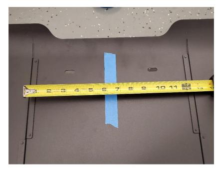
**2.27.** Place the differential cooler duct onto the Verus Engineering diffuser using the mark you just made as a reference for the center hole on the differential duct. The leading edge of the duct should be up against the leading edge of the diffuser (towards the front of the car).
