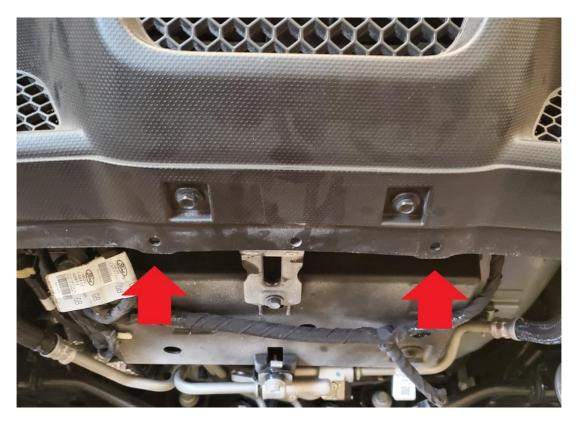
**2.13.** Drill these out to 3/8" if needed. Follow the instructions in the picture below to install the two M6 rivet nuts.
