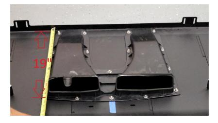
**2.26.** Measure the center of the Verus Engineering diffuser by using the two center strakes. Place a piece of tape, and make a line going towards the front of the diffuser. This line will help you center the differential duct on the diffuser.
