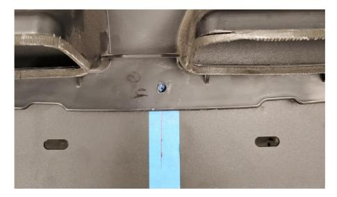
**2.28.** Mark, and center punch all of the holes for the differential duct, and drill them using the 1/4" drill bit. Again, it is recommended that you use touch up paint on all the raw edges.
