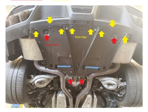
2.5. Below is a closer picture of where the three mounting brackets will go. The bolt circled in red will be the mid-bracket, the bolt circled in blue will receive the front bracket, and the holes circled in yellow will receive the outer bracket.
