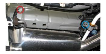
**2.8.** Install the front brackets as shown below. You can fully tighten the bolt back into the sway bar mounting location at this time. You may need to clearance the mounting ears to fit the sway bar bushing mount shown below.
