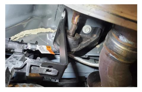
**2.11.** Install the outside brackets by using (2) of the M6 x 1.0 x 16mm long BHCS, (2) fender washers, and (2) nuts on the top side. The long slotted holes should be the holes being bolted here. This should look like below after **loosely** installing the brackets. They do not need to be tightened yet. Install the other side in the same manner.
