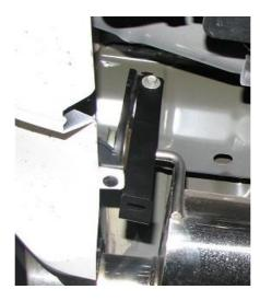
**2.10.** Slide an M6 fold nut onto the slotted hole on both mid-brackets.
