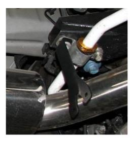
**2.9.** Install the mid-brackets as shown below. Note that there are a left-hand and a right-hand mid-bracket. The bottom of the bracket should angle upward in the rear. It is normal for the bracket will need to be slightly bent around the exhaust hanger.
