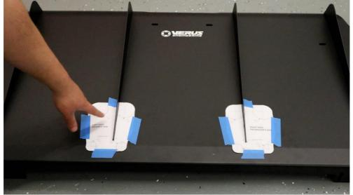
**2.18.** Center punch all of the holes to be drilled out.
