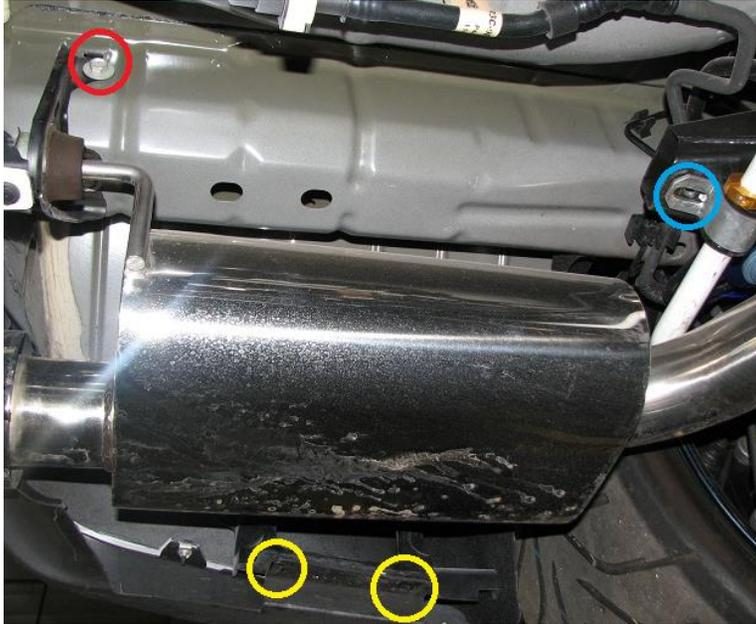
2.6. Starting with the outside mounting points, remove the two plastic clips. These are circled in yellow below. Use a screwdriver to remove these.
