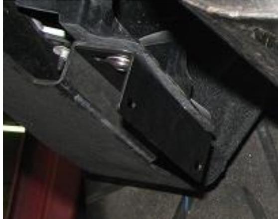
**2.12.** We will be installing two M6 rivet nuts into the holes shown below.
