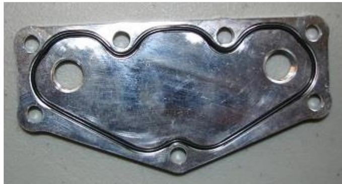
**4.2.** With the o-ring installed, we can install the plate onto the AOS with the (4) M6x1.0 x 16mm BHCS and M6 washers. You will also have to install the bracket at this time as shown in figure 4.3.
