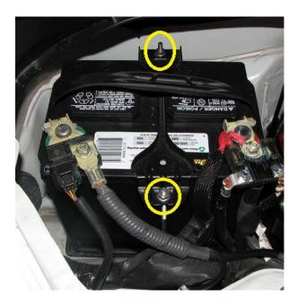
**2.4.** Fully remove the battery from the engine bay. With the battery out of the way, you will see a black plastic tray. Remove this as well which is shown in the below photo.
