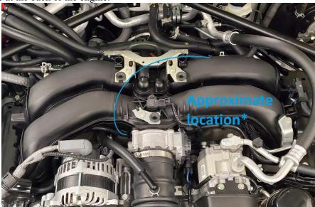
**4.6.** This will expose two barbs (one on the throttle body, and one on the coolant pipe) that we can use for the coolant circuit.
