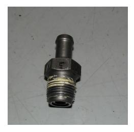
**2.8.** Install the supplied 3/8NPT to 1/2" adapter fitting. You will need a 7/8" deep socket to install this. It is recommended to use some Teflon tape or sealant to ensure a leak free seal as shown below. Install this adapter to 12-18 ft-lbs.
