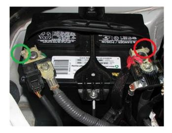
**2.3.** To fully remove the battery, loosen the 10mm nuts on the top of the two studs circled in yellow below. The j-hook studs will then come off the chassis and you can fully remove the tie-down.
