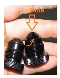
**3.3.** Then, install the black 6AN to 1/2" barb into this and torque to 8 ft-lbs. A photo of this is shown below. When installing the black 6AN to 1/2" nipple, do so with the knurled fitting already installed on the AOS.
