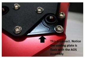
**3.3.** With the bracket, AOS, and coolant add on plate bolted together we will need to install the banjo fittings. Currently snug these down so that the barbs stay in place, do not torque them down at this time. Use the picture below as a guide for the correct clocking of the banjo fittings. For reference, the barbs are pointing towards the driver side on a USDM car.
