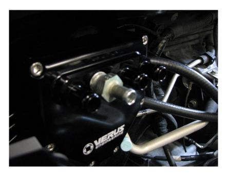
2.13. Now it is time to run the hoses. We will be using the PCV valve, and the 1/2" hose barb on the passenger side of the PCV valve. The hose routing will look something similar to what is shown below. \*\*Important: Our hose routing may differ from what works best with your set up. ALWAYS verify the correct hose length before cutting.\*\*
