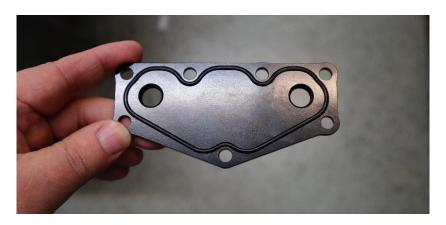
3.2. Once the o-ring placement is verified, place the cooling plate onto the AOS assembly. Place the mounting bracket on top of that and use seven 16mm long M6 BHCS with washers to bolt the three pieces together. Torque to 6 ft-lbs. \*\*Make sure the o-ring does not get pinched when tightening the bolts down.\*\*
