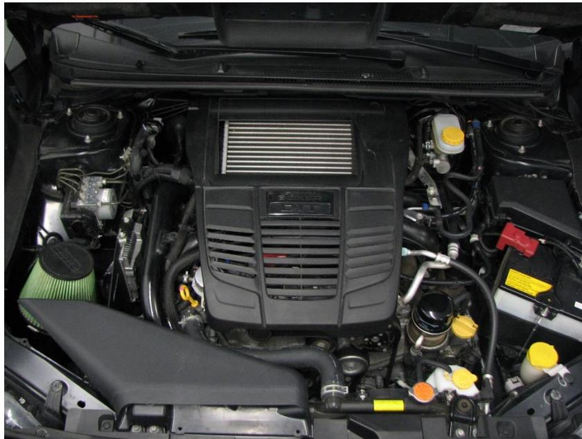
**2.3.** For this install, we have to remove the intercooler if you still have a TMIC (Top Mount Intercooler). Start by removing the **(2) 12mm bolts** that hold the intercooler down.
