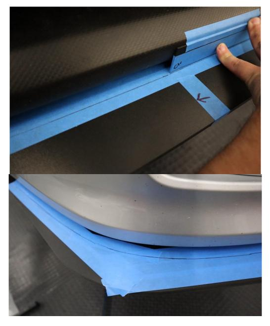
**2.7.2.** Once the outline is traced onto the splitter, transfer the marks made in step 2.4 onto the splitter.
