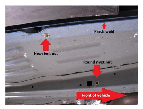
**2.6.2.** Using the instructions below, install the hex-rivet nut into the center of the square hole.
