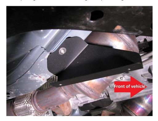
**2.6.** Next, we will be installing two rivet nuts, one hex-rivet nut, and one round rivet nut.
