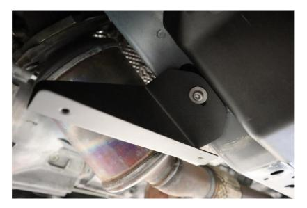
**2.9.** Install the driver side middle bracket using the existing "nut" as shown. It is the forward-most "nut" of the two on the car. This should come off by hand, however a 23mm socket can help with removal and installation. Tighten only by hand.
