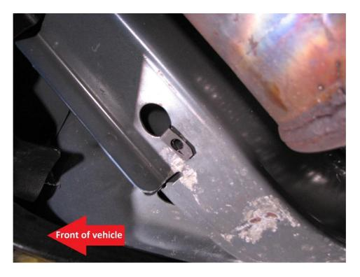
**2.5.** Install the passenger side front bracket making sure it points straight ahead as shown.
