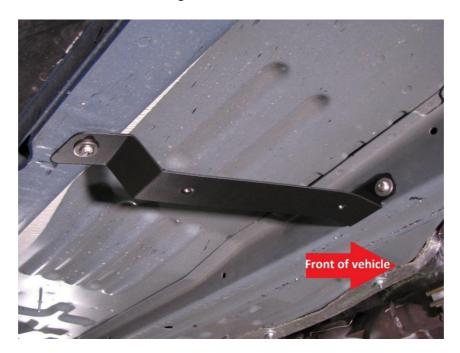
**2.7.** Install the passenger rear bracket parallel with the fuel tank as shown. Use a 13mm socket, and the existing nut on the vehicle. Tighten to 13 ft-lbs.
