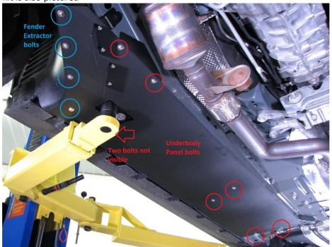
**2.12.** At this point you may choose to install some strips of foam tape between the underbody panel and the frame rails. The panels did not rattle on our test vehicle however the potential is still there. This is purely optional.
