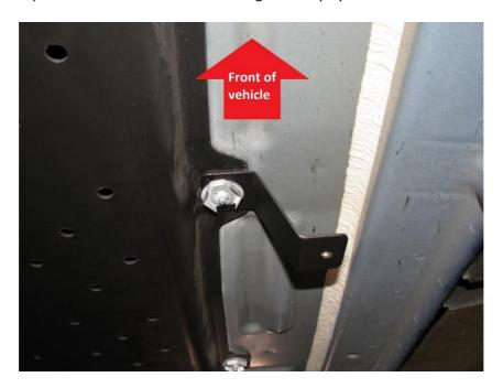
**2.9.1.** Install the driver side rear bracket using the existing 13mm-head nut. Align the bracket parallel with the fuel tank. Tighten to approximately 13 ft-lbs.
